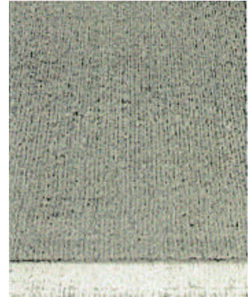
13 mm Uniform Transverse ETD = 1.793, d = 2.2, w = 6.2
