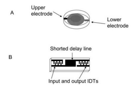
Schematic representation of: A) TSM resonator and B) SH-SAW device platforms. Only a single delay line is shown on the SH-SAW substrate.
