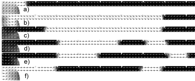
Fig. 4. Static and dynamic pinning allows for precise control of a domain wall. Walls can be injected (a), driven past notches (b) and placed where you want them as other walls are injected into the wire (c). Figs. (d)–(f) show three different final domain wall configurations which could be considered bit sequences.
