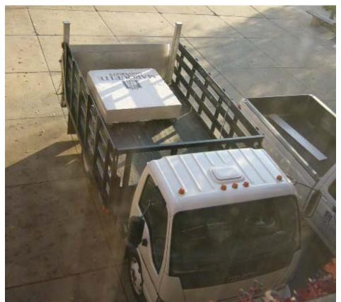
Figure 3-28 - Vehicle used to calibrate the WIM system. Note the concrete slab placed in the bed of the truck over the rear axle.
