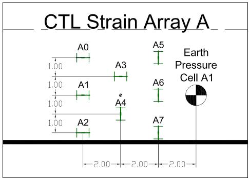
Figure 3-13 - Spacing of the strain gauges and earth pressure cells are shown above. All units are in feet. Note that the orientation of the two gauges in the middle of the array alternate rotation angles (transverse vs. longitudinal) for the two CTL arrays as shown in Figure 3-14.
