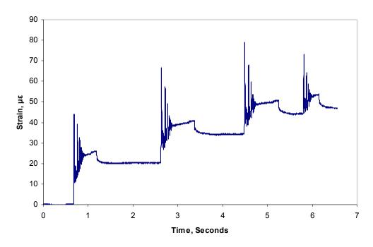
Figure 3-33 – CTL gauge B1 strain response to an impulse loads generated from and FWD.
