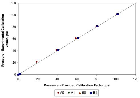
Figure 3-8 - Earth pressure cell calibration data.
