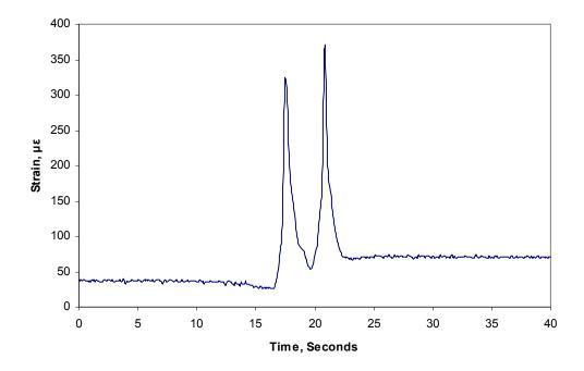
Figure 3-29 - Dynatest PAST II - AC gauge C4 response to roller pass.
