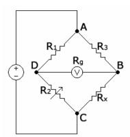
Figure 3-2 - Wheatstone Bridge circuit.
