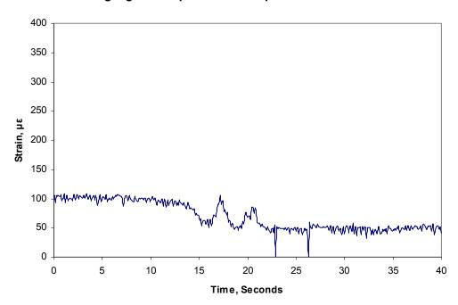
Figure 3-31 –Dynatest PAST II – AC gauge C7 output. Although not explicitly clear, this sensor has a substantial amount of signal noise compared to similar gauges.
