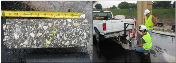
Figure 3-38 – Left: Core sample removed from the pavement. Right: The core-drill was secured against the weight of a vehicle to produce samples with very smooth side walls for possible future testing.
