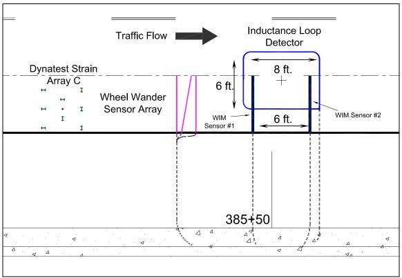
Figure 3-17 - Layout of the WIM sensors (loop detector and two quartz piezo strips) and the wheel wander sensors. The conduits installed into the pavement are also shown as hidden lines extending from the instruments to the curb.
