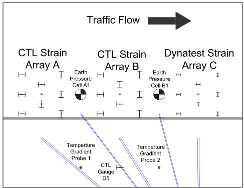
Figure 2-1 - Layout of the three strain gauge arrays, earth pressure cells, and pavement temperature gradient probes.
