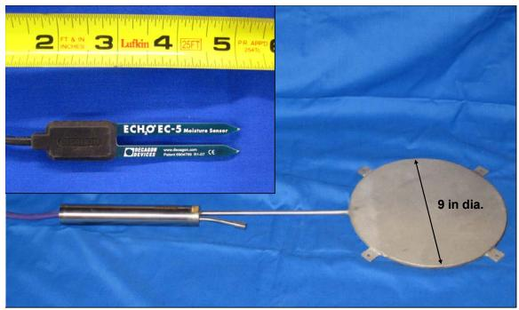
Figure 3-7 - Geokon earth pressure cell and Decagon soil moisture probe.
