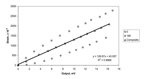
Figure 3-4 - Example of calibration data.
