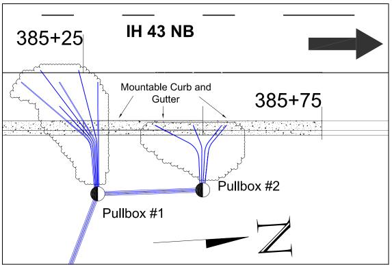
Figure 3-35 – The conduits within the cloud are those installed for the strain sensors, base EPCs, WIM and Wander components.
