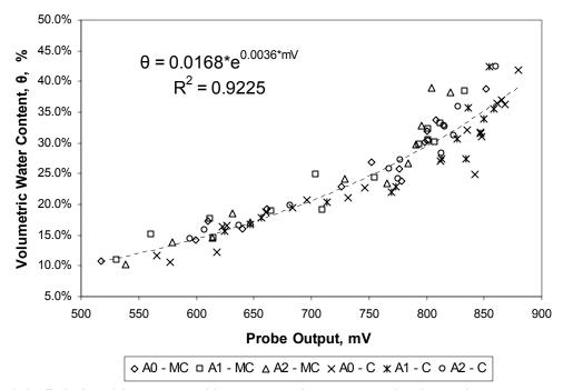
Figure 3-9 - Relationship generated between probe output and volumetric water content ( $\theta$ ) for three probes and two different soil types. The probes and soil type are designated respectively as A0, A1 and A2; and MC (silty-clay) and C (clay).
