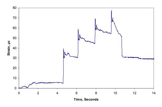
Figure 3-32 – CTL gauge A0 strain in response to a series of four Marshall Hammer drops in succession.
