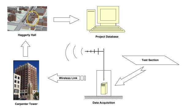
Figure 4-1 – Data transmission path.
