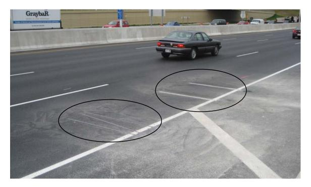
Figure 3-27 – Test section opened to traffic with the wheel-wander and WIM sensors installed (circled areas).
