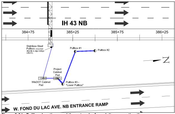
Figure 3-34 - Pullbox locations and the network of conduits connecting them.
