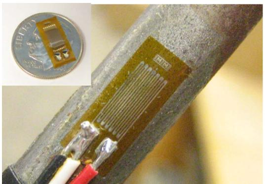
Figure 3-1- Bonded electrical resistance strain gauge mounted to a steel rod.
