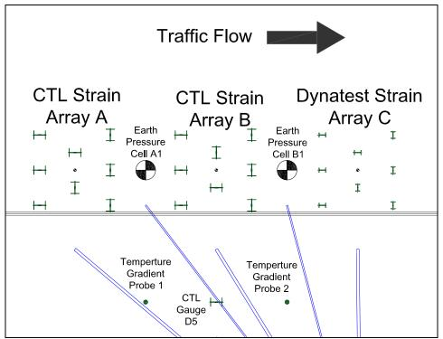
Figure 3-14 - Final configuration of strain gauges, earth pressure cells, and pavement temperature gradient probes.
