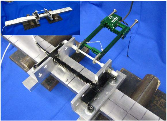
Figure 3-6 - Test setup for calibration of the Dynatest gauges.
