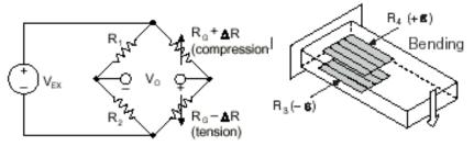
Figure 3-3 - Circuit diagram and physical arrangement for the half-bridge circuit.
