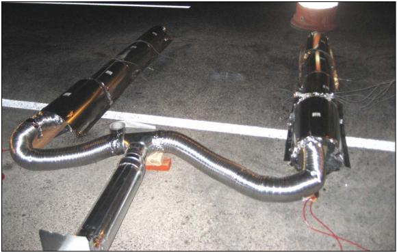
Figure 3-25 - The heating assembly was placed over the two slots cut for the WIM sensors. Heat was supplied by a forced-air kerosene fueled heater (not pictured). The sections of the assembly were sealed with aluminum ducting tape to minimize heat loss. Multiple temperature probes were in place to accurately measure pavement temperatures.
