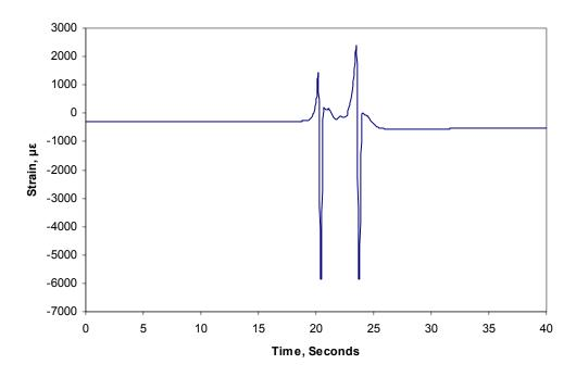
Figure 3-30 – CTL ASG gauge B0 response to roller pass.
