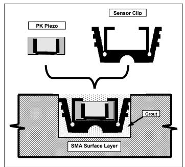
Figure 3-23 – Cross section of the PK piezo strip used for the wheel wander grid showing how it is assembled in the pavement.
