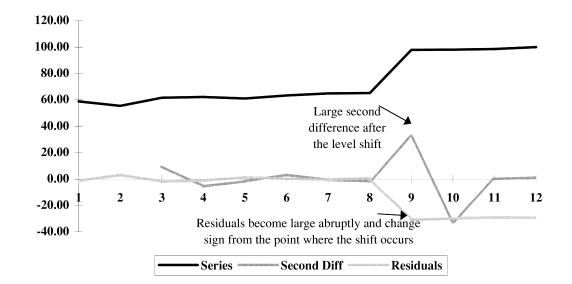
Figure 2: Detecting a Level Discontinuity: An Example
