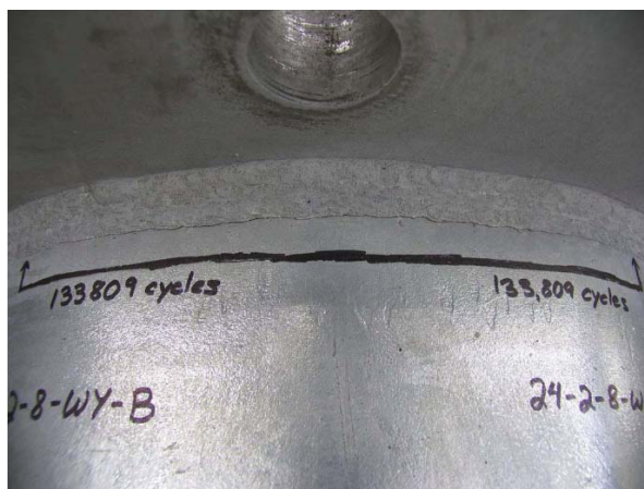
Figure 5.3: Typical failure of Wyoming full penetration weld connection
