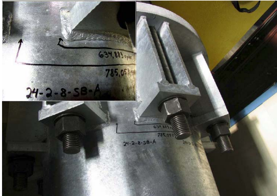
Figure I.5 Stool Base Specimen Fatigue Failures Seen in Testing (Rios 2007).
