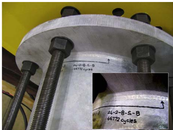
Figure 5.1: Typical failure of fillet welded socket connection
