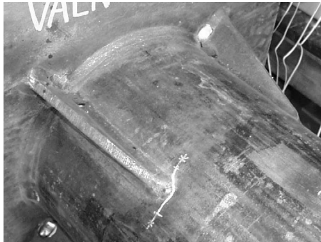
Figure G.6. Typical Fatigue Failure of 45-Degree Wedge-Type Stiffener Reinforced Connection (Koenigs et al 2003).
