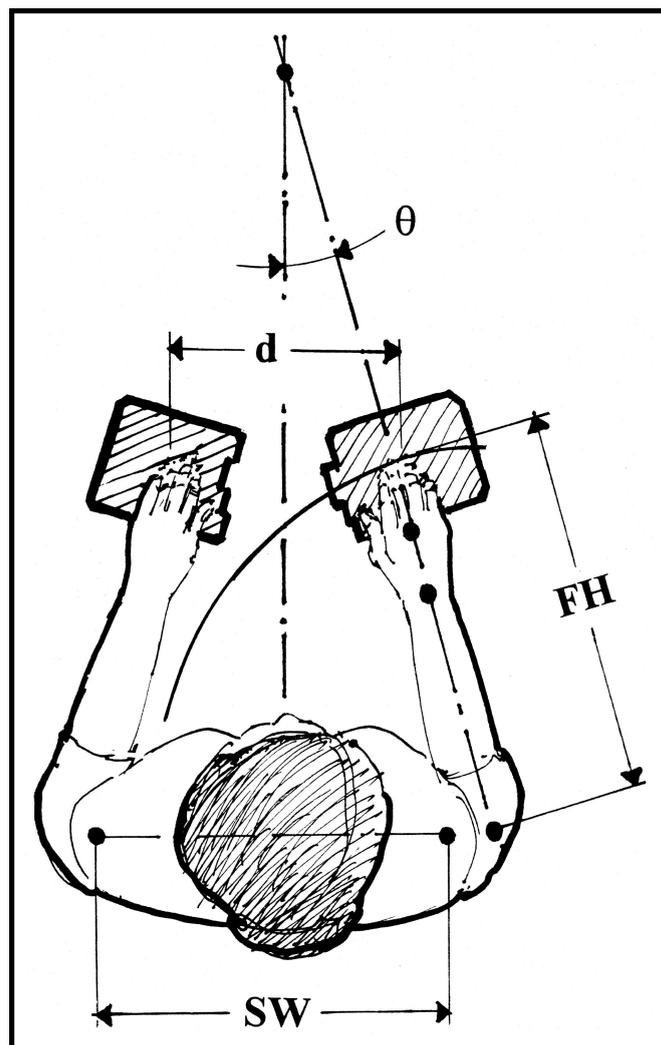
**Figure 5.** Geometric model for establishing slant angle of each keyboard half. SW=shoulder width, FH=forearm-hand length, d=distance between the centers of both keyboard halves,  $\theta$ =slant angle of each half of the keyboard.
