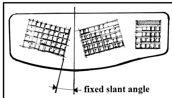
**Figure 1.** Drawing of a typical split computer keyboard. This keyboard has a fixed opening angle of 25 degrees, resulting in a slant angle of 12.5 degrees for each keyboard half.
