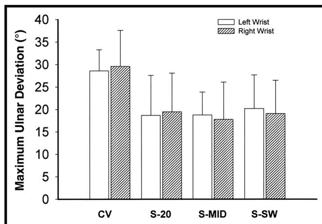
**Figure 7.** Maximum wrist ulnar deviation of the left and right wrists for the 4 keyboard configurations. The values plotted are the averages of the maximum data across subjects. Bars represent 1 standard deviation. See Figure 2 caption for explanation of abbreviations of keyboard configurations.
