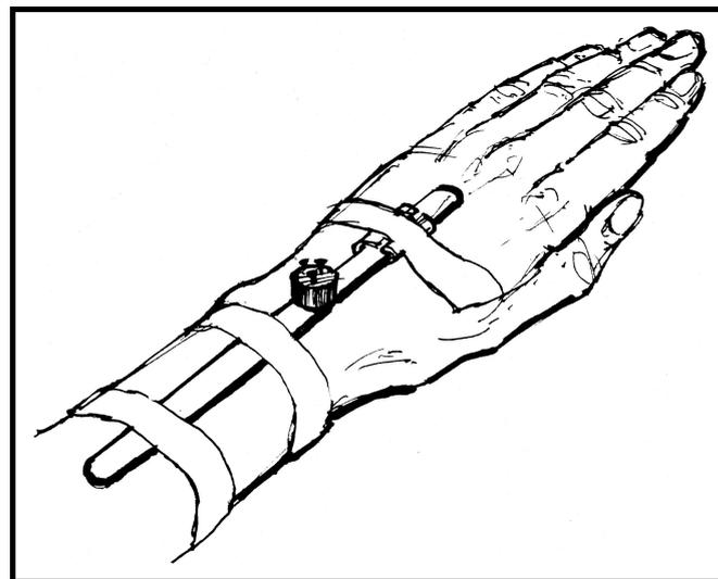
**Figure 4.** Wrist monitor that measured wrist radial and ulnar deviation.
