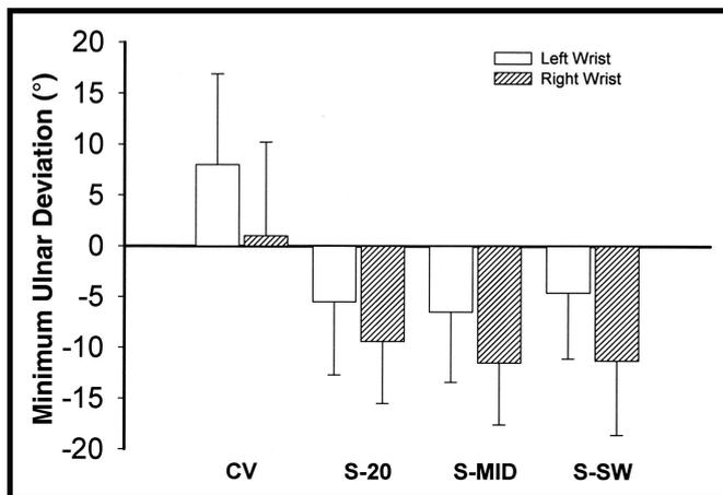
**Figure 8.** Minimum wrist ulnar deviation of the left and right wrists for the 4 keyboard configurations. Ulnar deviation angles are plotted as positive, and radial deviation angles are plotted as negative. The values plotted are the averages of the minimum data across subjects. Bars represent 1 standard deviation. See Figure 2 caption for explanation of abbreviations of keyboard configurations.
