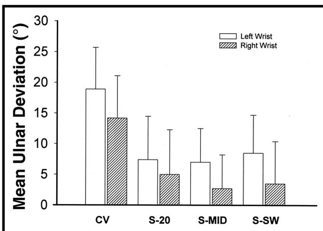
**Figure 6.** Mean ulnar deviation of the left and right wrists for the 4 keyboard configurations. Bars represent 1 standard deviation. See Figure 2 caption for explanation of abbreviations of keyboard configurations.
