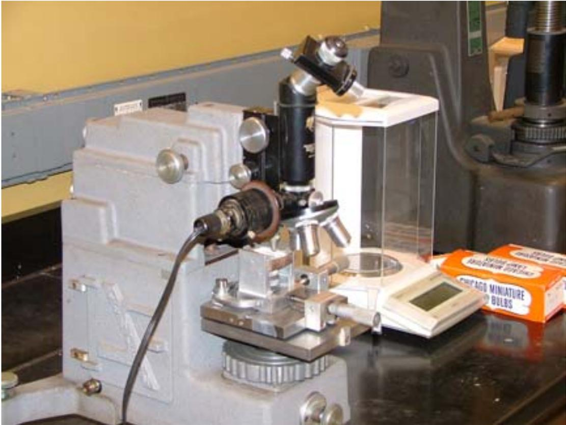
Figure 3. Close-up View of Metal Block with MTA in Vickers Tester
