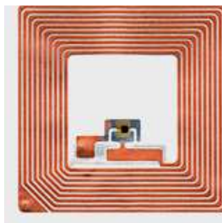
Figure 1.1: An RFID tag (source: http://www.barcode-solutions.com )
