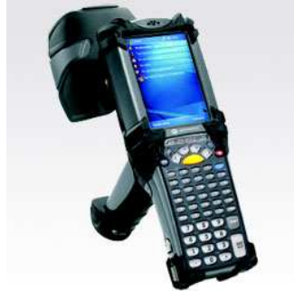
Figure 1.2: An RFID reader (source: http://www.barcode-solutions.com )
