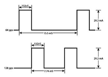
**Figure 4.** Waveform of LVMPC used in several clinical trials<sup>12,17,18,20</sup> that reported positive healing outcomes after treatment of chronic wounds in conjunction with standard care. LVMPC, low-voltage monophasic pulsed current.
