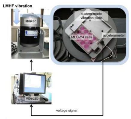
**Figure 1:** A rigid vibration plate was custom-made to fit two standard multi-well tissue culture plates. LMHF vibration was delivered through a vibration shaker controlled by a feedback loop consisting of an accelerometer attached to the vibration plate and a computer equipped with a VibeLab user interface.
