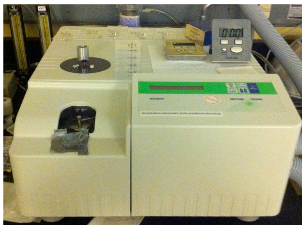
Figure 1. Mettler Toledo DSC used for measuring heat flow
