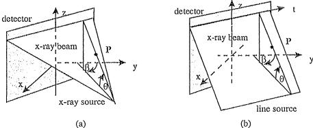
Fig. 2 different sampling geometry (a): cone beam (b) tilted parallel beam
