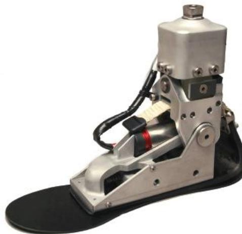
Figure 1.7 Original PowerFoot One by iWALK Company [14]
