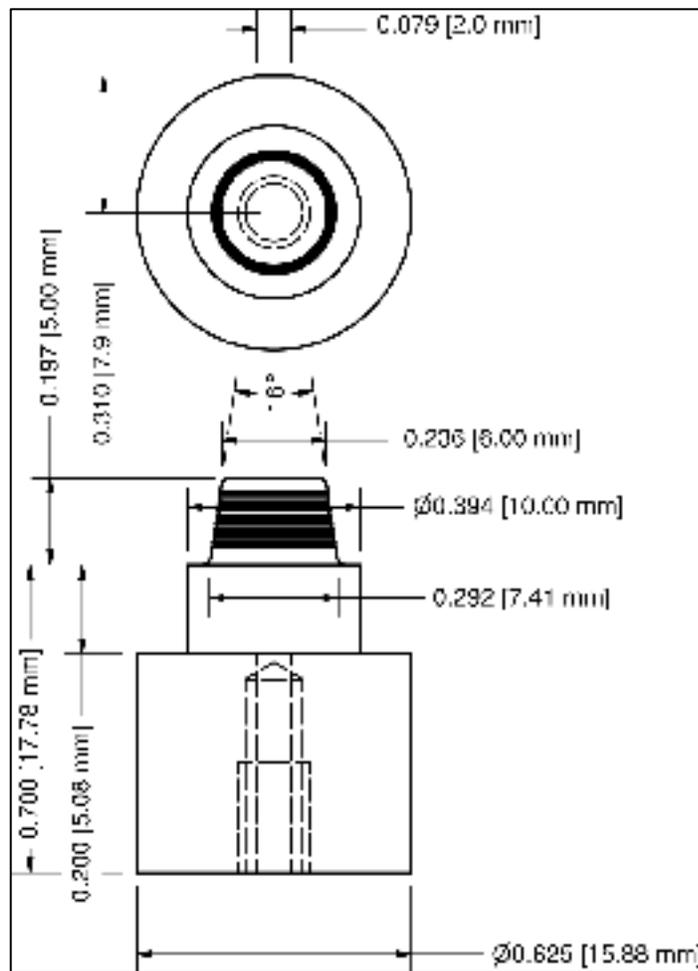
Figure 1 – Dimensions of dies
