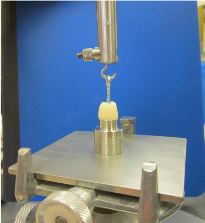
Figure 6 – Attaching hook to provisional crown
