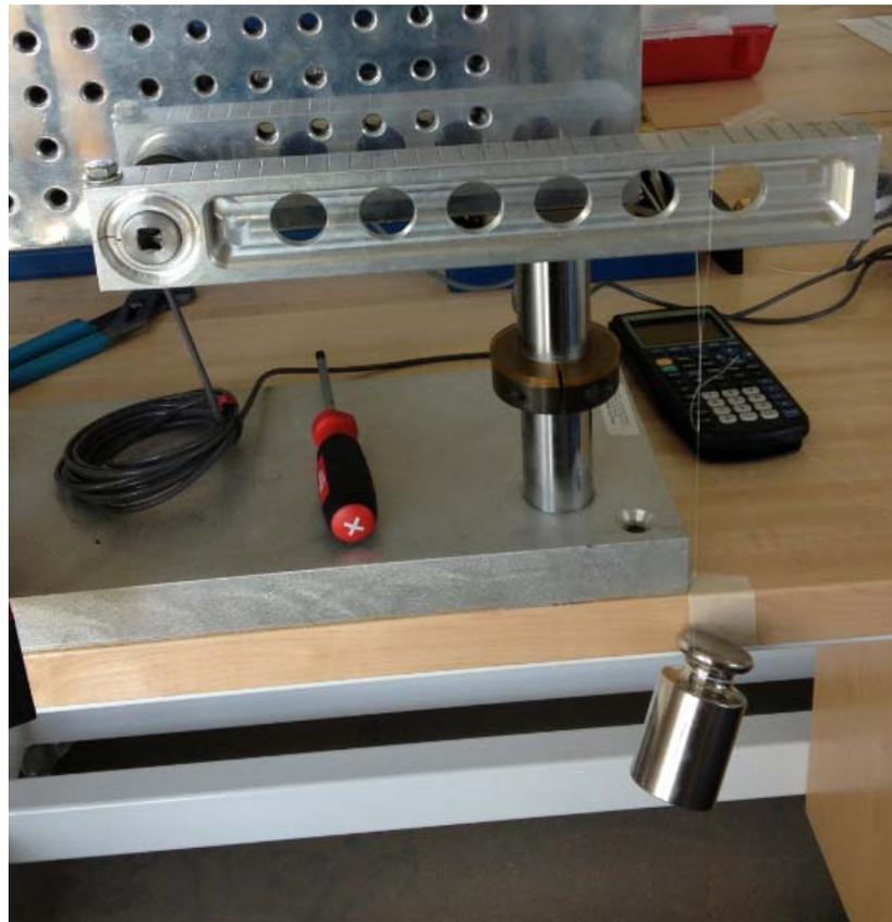
**Fig. 3.12: Torque Load Cell Calibration.**
