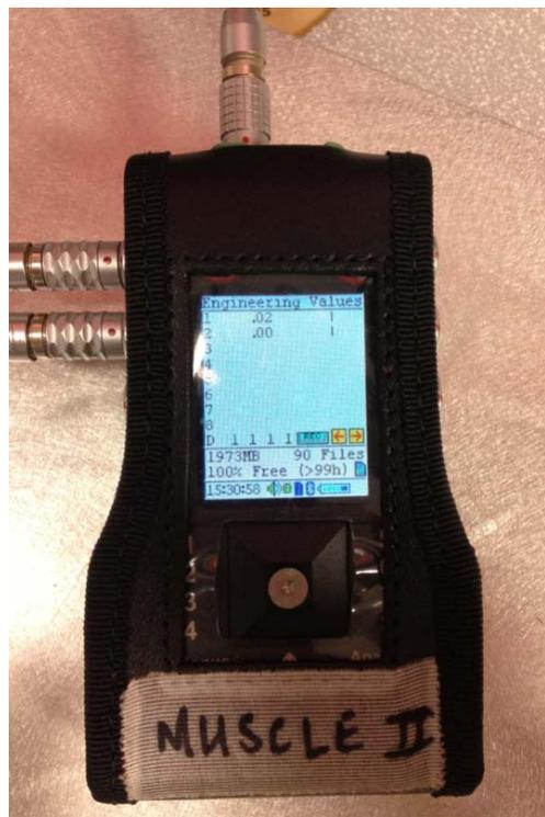
**Fig. 3.9: Biometrics Datalog Wireless Data Unit**
