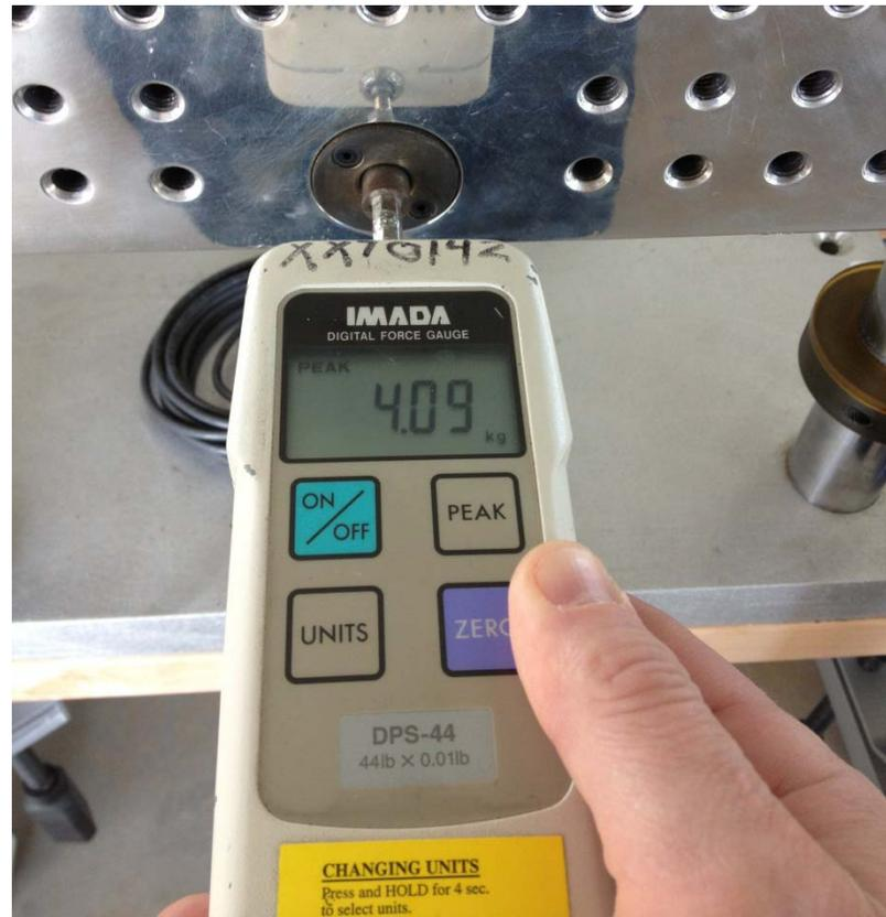
**Fig. 3.14: Axial Load Cell Calibration**
