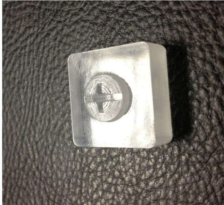
**Fig. 3.8: SLS Model of Test Specimen**
