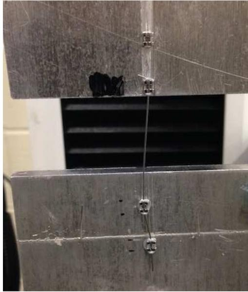
**Figure 8.** Photo of testing setup after test was run, illustrating bracket offset and terminal bend of wire. The upper plate had a groove with 4 brackets mounted to it. The lower modified plate was cut into two pieces. The white layer was the PDL replica that allows for physiological mobility of the upper test bracket.
