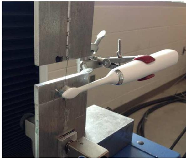
**Figure 11.** Sonicare tooth brush directly placed against test bracket/wire interface.
