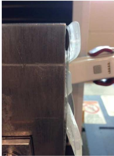
**Figure 9.** Bite force sensor and AcceleDent unit
