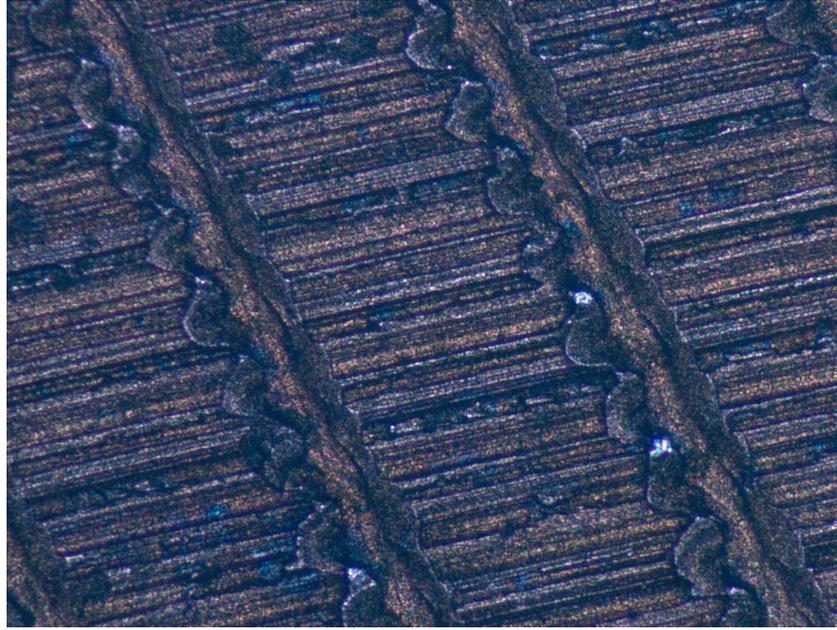
Figure 3.5 - Close up view of the grooves on the 125  $\mu\text{m}$   $R_a$  die after machining. The magnification is 400x.
