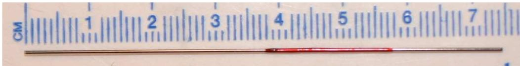
Figure 2. Wire isolated with nail polish
