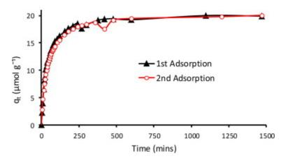
Fig. 7. Plot of  $q_t$  of adsorption of 2,4,5-TCP as a function of time by 30:20:50 CEL:CS:B15C5 composite film: Black curve is for 1st adsorption (i.e., by freshly prepared films) and red curve is for 2nd adsorption (i.e., adsorption by films that were regenerated by desorbing 2,4,5-TCP previously adsorbed). (For interpretation of the references to color in figure legend, the reader is referred to the web version of the article.)
