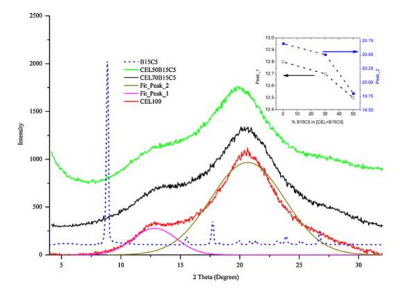
Fig. 3. XRD spectra of B15C5 powder (blue dashed line), 100% CEL film (red), 50:50. CEL:B15C5 film (green) and 70:30 CEL:B15C5 film (black). Insert is plot of  $2\theta_{max}$  value for resolved band at 12.8° and 20.7° as a function of B15C5 concentration in the composites. (For interpretation of the references to color in figure legend, the reader is referred to the web version of the article.)
