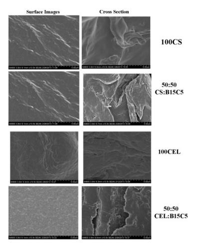
Fig. 4. SEM images of surface (left images) and cross section (right images) of regenerated films of 100% CS (top row), 50:50 CS:B15C5 (2nd row), 100% CEL (third row) and 50:50 CEL:B15C5 (bottom row).
