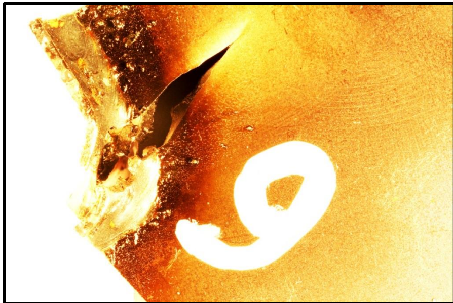
Figure A9. Photo of the crack sectioned at the end of test of Specimen 6.
