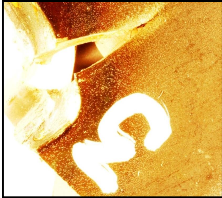
Figure A6. Photo of the crack sectioned at the end of test of Specimen 3.
