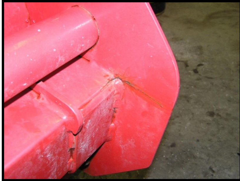
Figure D1. View of a typical field failure (inner surface of rib)
