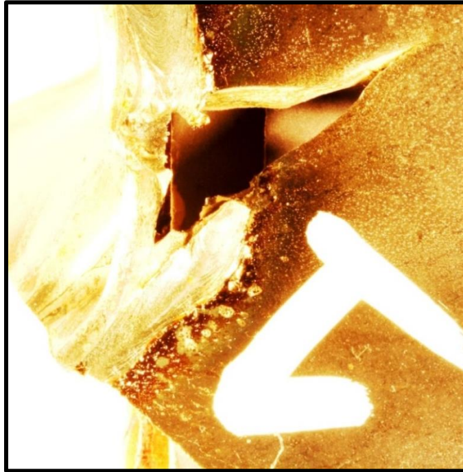
Figure A4. Photo of the crack sectioned at the end of test of Specimen 1.
