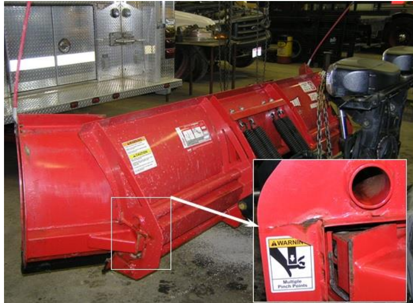
Figure 1. View of the snowplow and the fatigue failure site location.
