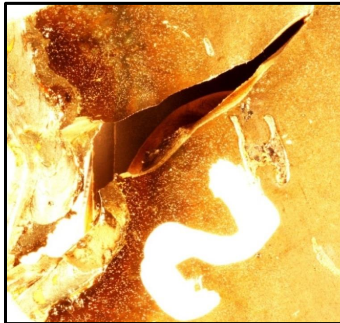
Figure A5. Photo of the crack sectioned at the end of test of Specimen 2.
