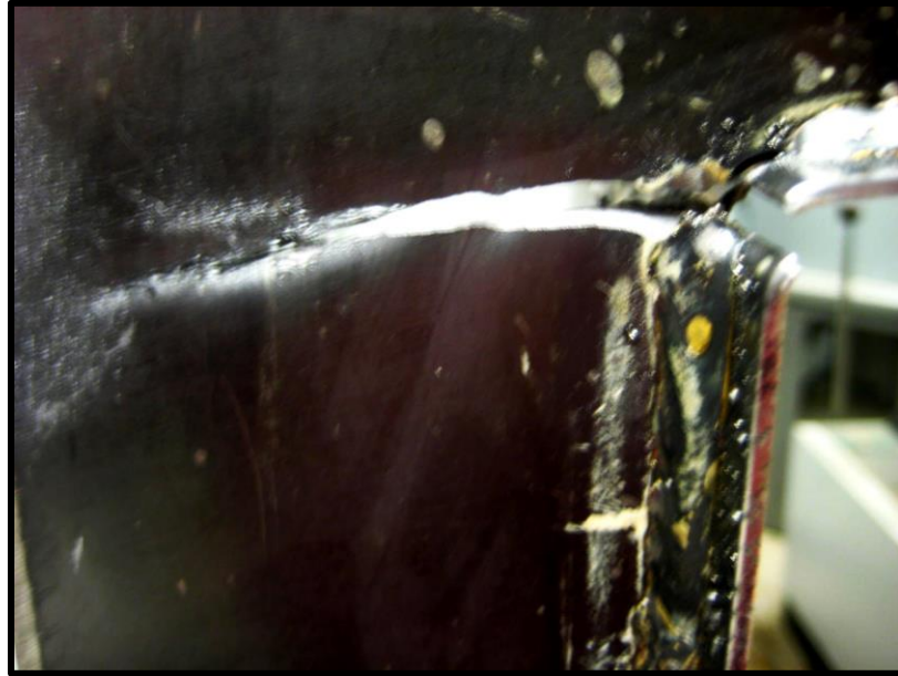
Figure A1. Photo of the final crack length of a test specimen.
