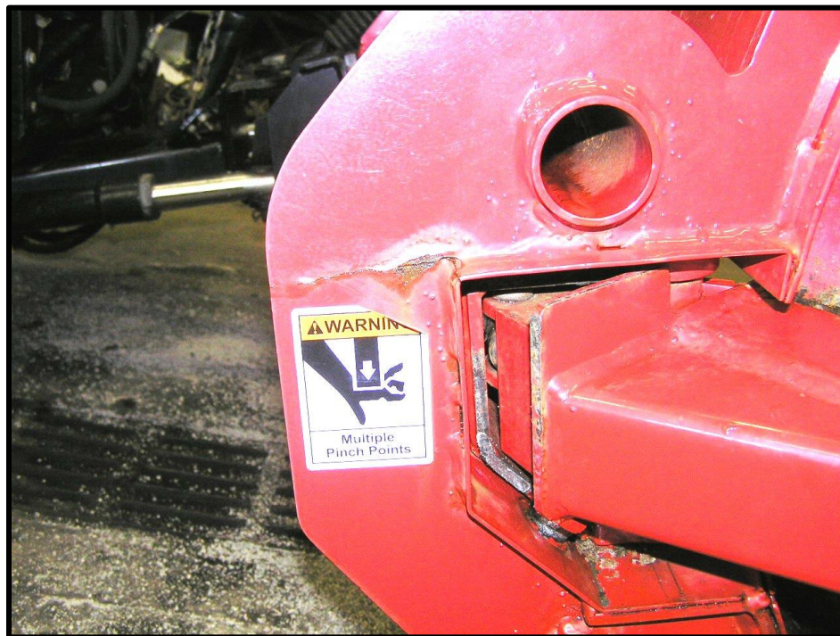
Figure D4. View of a typical field failure (outer surface of rib).
