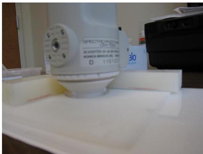
**Figure 10. Spectrophotometer placement on holder.**
