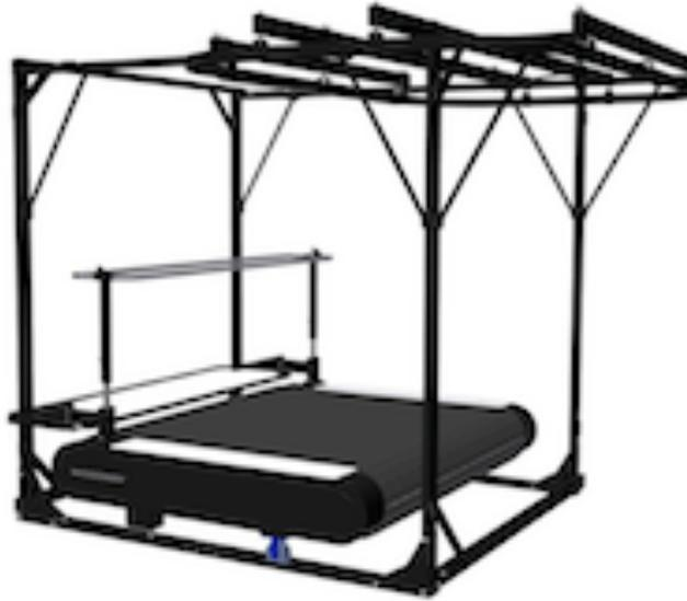
Figure 2. Blade skating treadmill with overhead gantry system. Adapted from [19].
