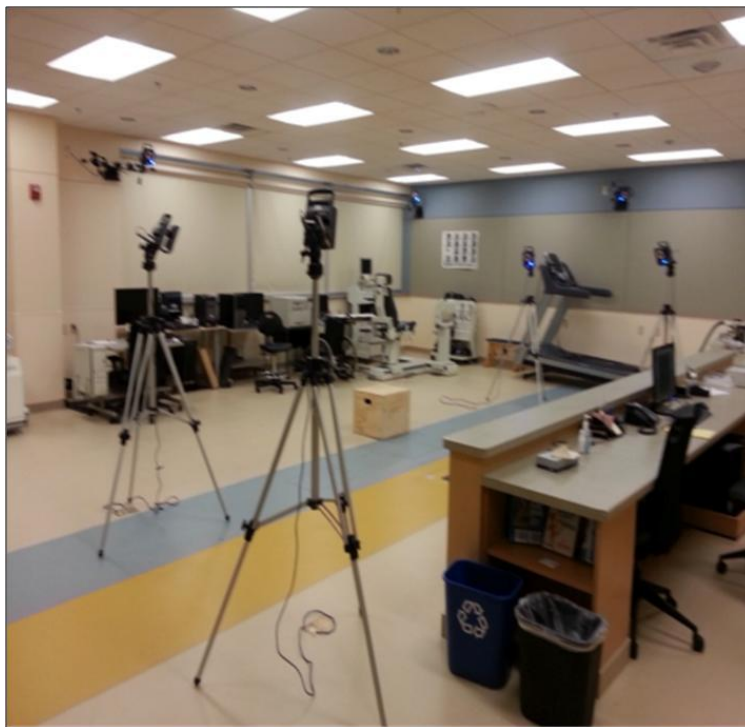
Figure 6: Motion Capture Laboratory Twelve Camera Setup with 30 cm plyometric box placed just behind floor-embedded force platforms.
