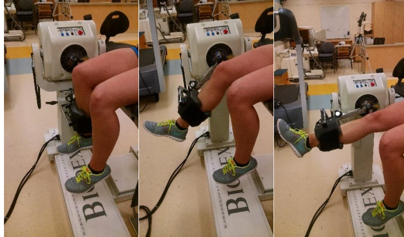
Figure 8: Biodex set up for knee flexion/extension at 90, 60, and 30 degrees of flexion
