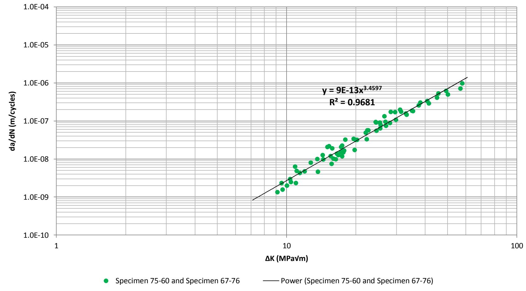
Figure H.11. Crack growth rate data and Paris Equation for AWS A5.28 at stress ratio  $R=0.05$  with a test frequency of 60Hz.
