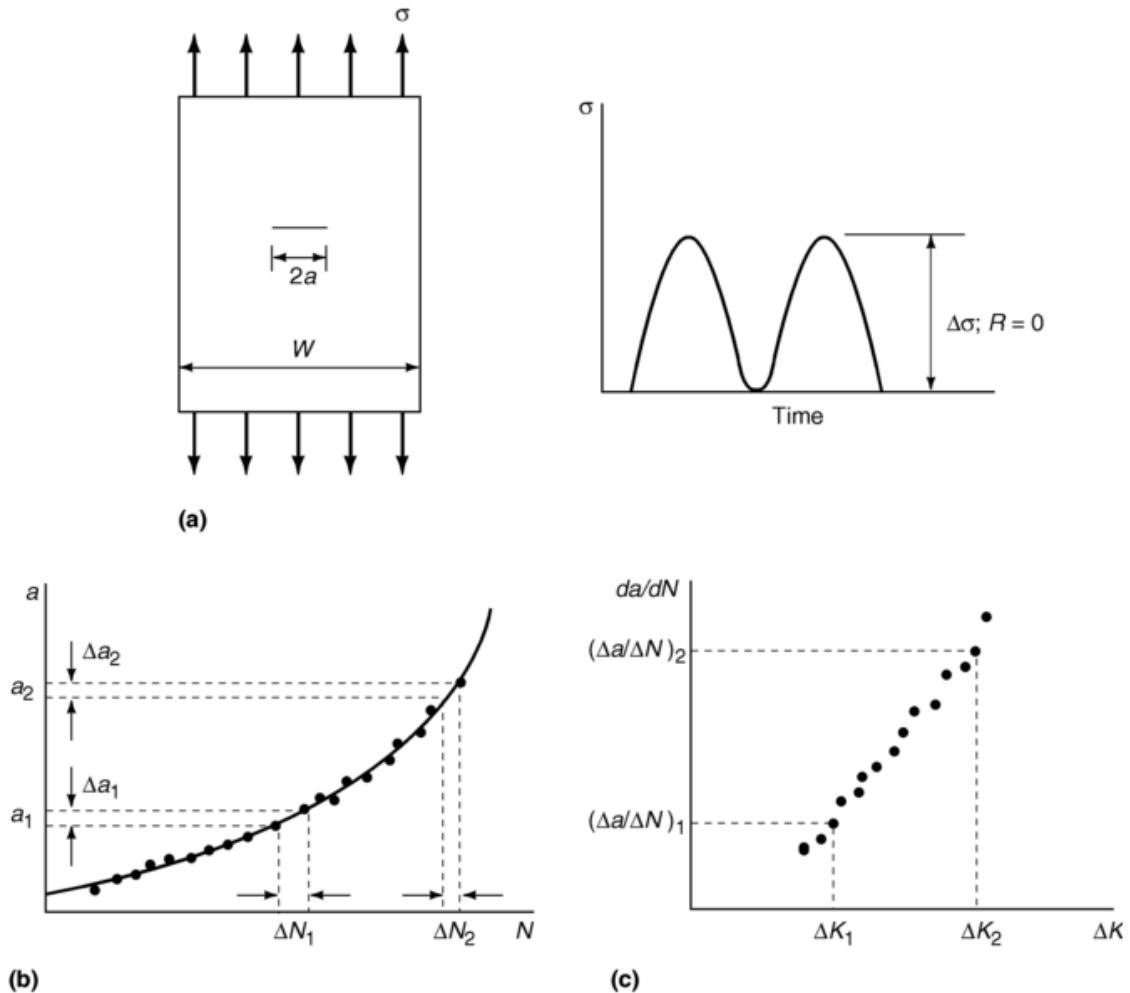
Figure 2.1. Schematic diagram of a middle tension test specimen, test data, and modeling process for generating fatigue crack growth data ( $\frac{da}{dN} - \Delta K$ ) data. (a) Specimen and loading. (b) Measured data. (c) Rate data. [2]
