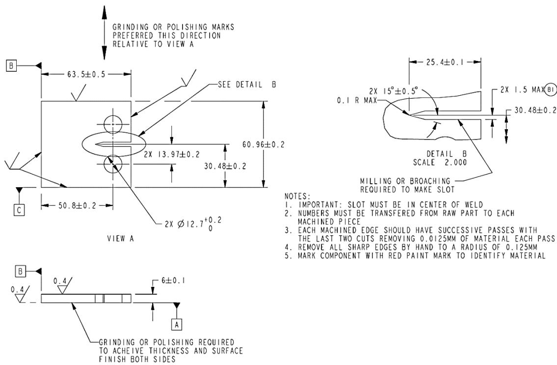
Figure 3.1. Specifications for machining compact specimen (units: mm)
