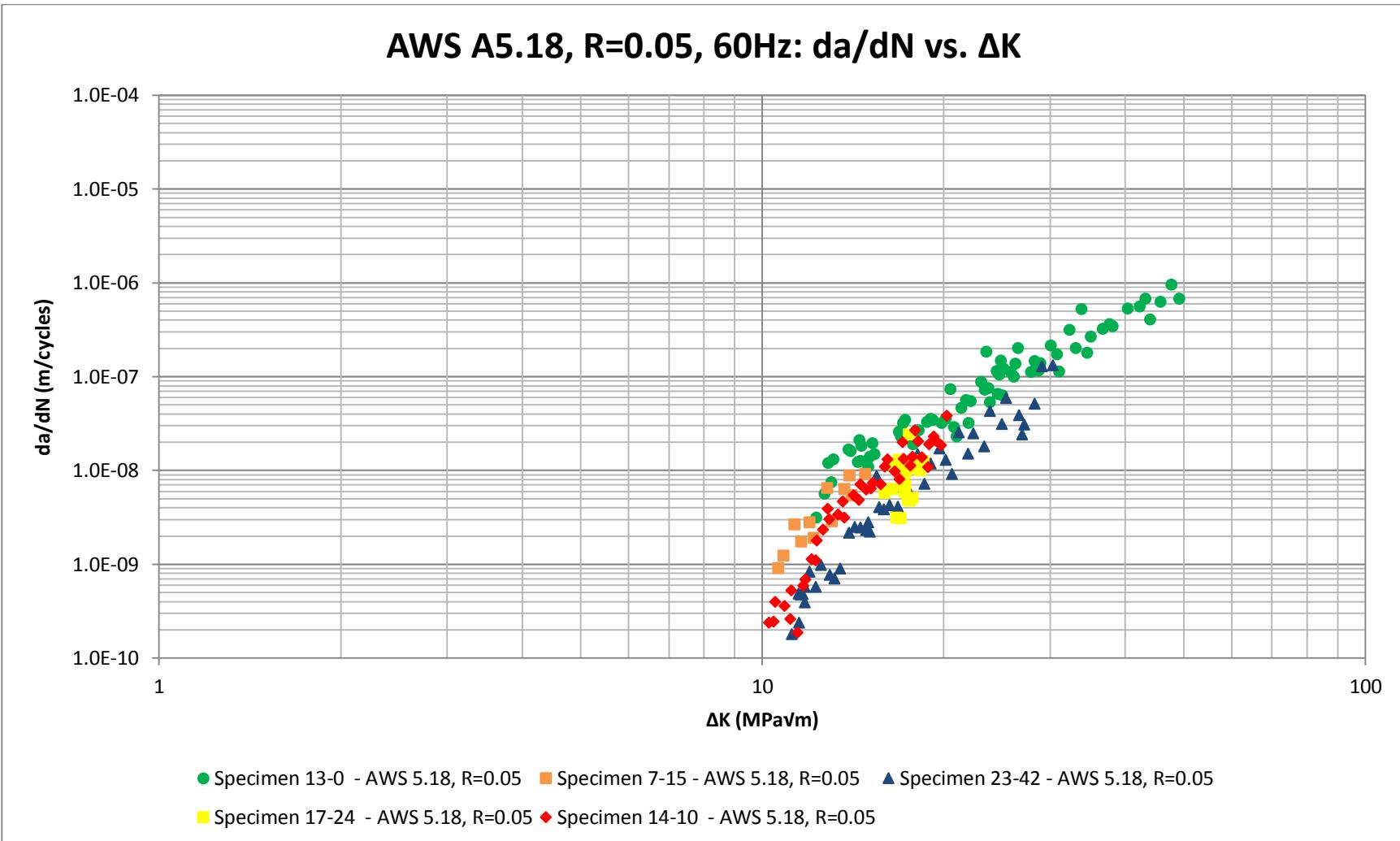
Figure H.5. Fatigue crack growth data for AWS A5.18 at stress ratio R=0.05 with a test frequency of 60Hz.
