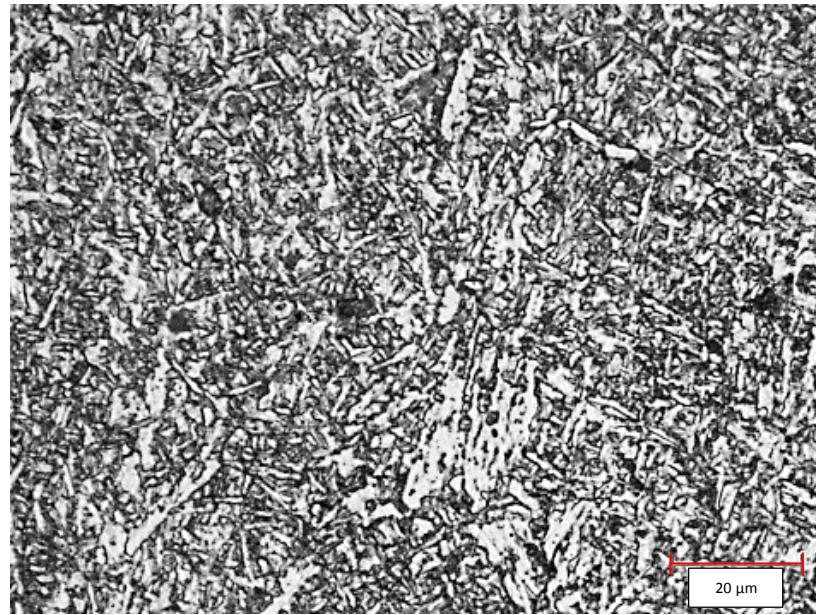
Figure 4.5. Image of etched AWS A5.28 weld metal specimen at high magnification showing it to consist of fine acicular grains of ferrite with some fine carbides.
