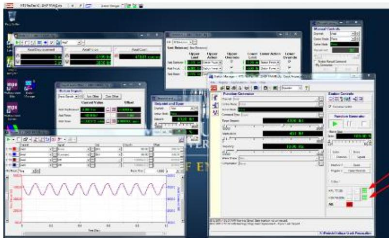
7. Start test. Monitor Axial Force and Axial Commanded Force for convergence (both traces should follow each other within several  $lb_f$ ).
