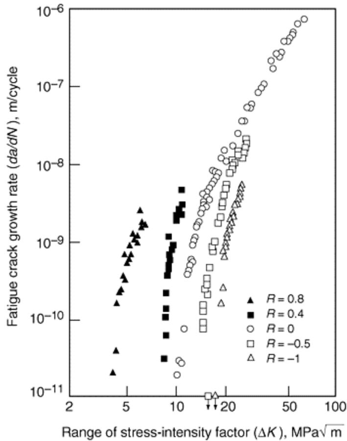
Figure 2.4. Comparison of load ratio ( $R$ ) effects on fatigue crack growth rate in JIS SS41 steel.
