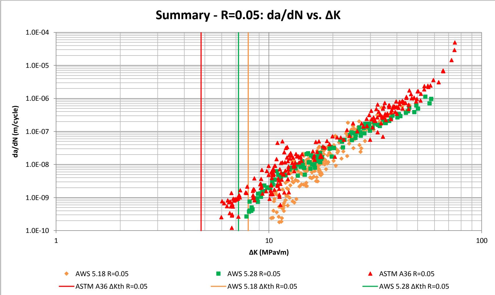
Figure 5.1. Summary of all fatigue crack propagation results for R=0.05.
