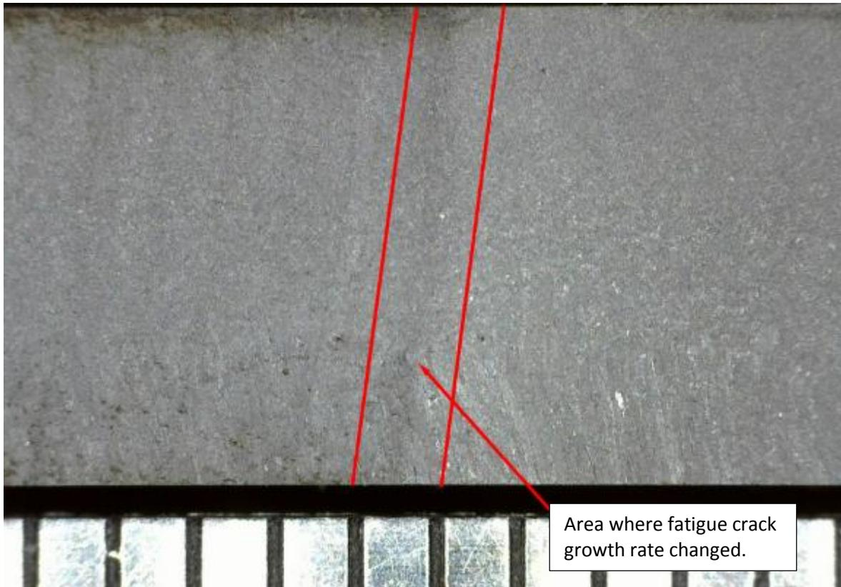
Figure 4.13. Fracture surface of AWS A5.28 material test Specimen #55-66. Measurement units are mm.
