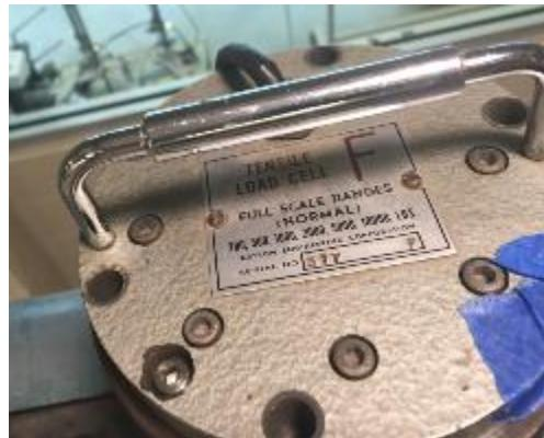
Figure B.2. 10,000 lb<sub>f</sub> load cell identification
