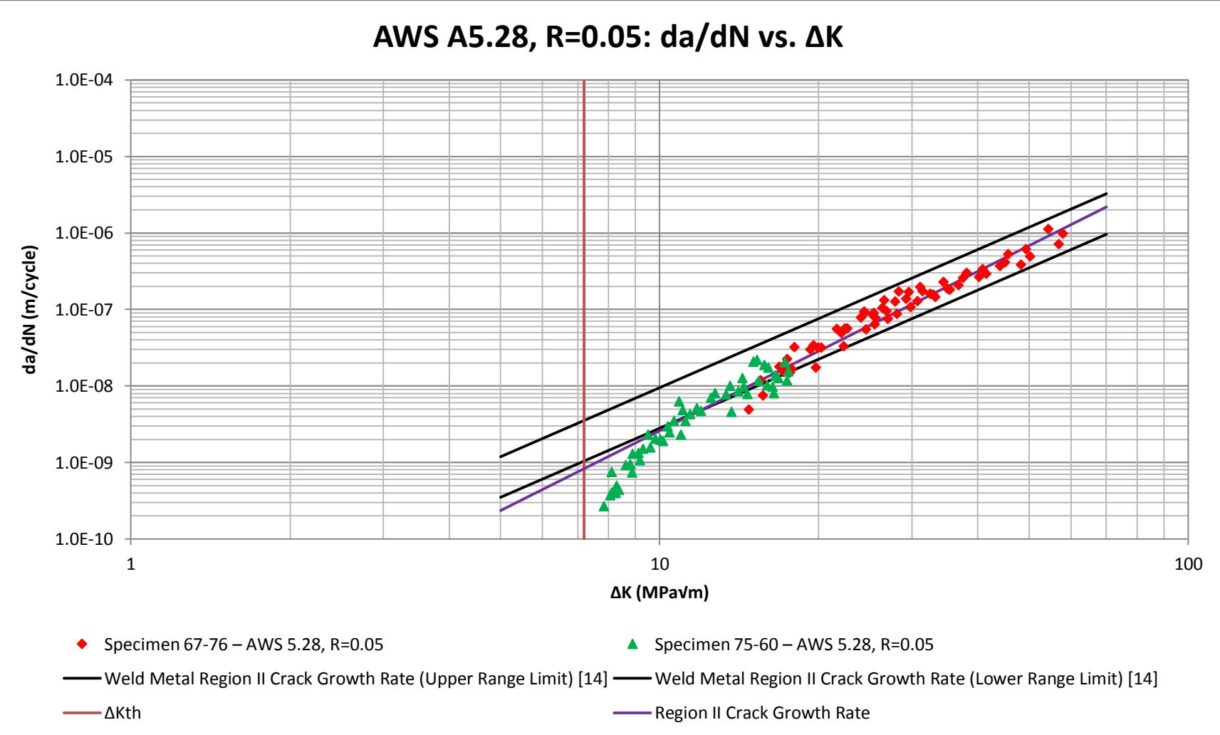
Figure 4.11. AWS A5.18 fatigue crack propagation results for R=0.05.
