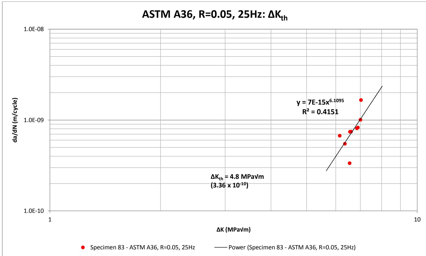
Figure 4.14.  $\Delta K_{th}$  data for ASTM A36 at stress ratio R=0.05 with a test frequency of 25Hz.
