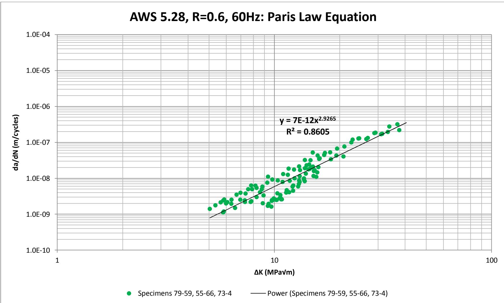
Figure H.13. Crack growth rate data and Paris Equation for AWS A5.28 at stress ratio R=0.6 with a test frequency of 60Hz.
