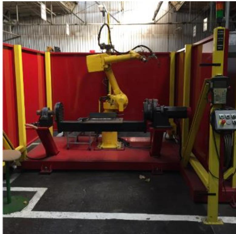
Figure 3.4. Vizient GMAW robot used for making the weld metal specimens
