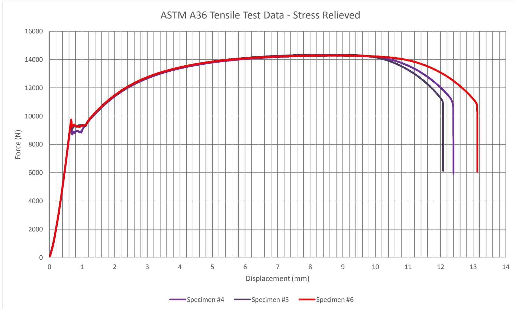
Figure C.2. Tensile test data of stress relieved specimens – ASTM A36
