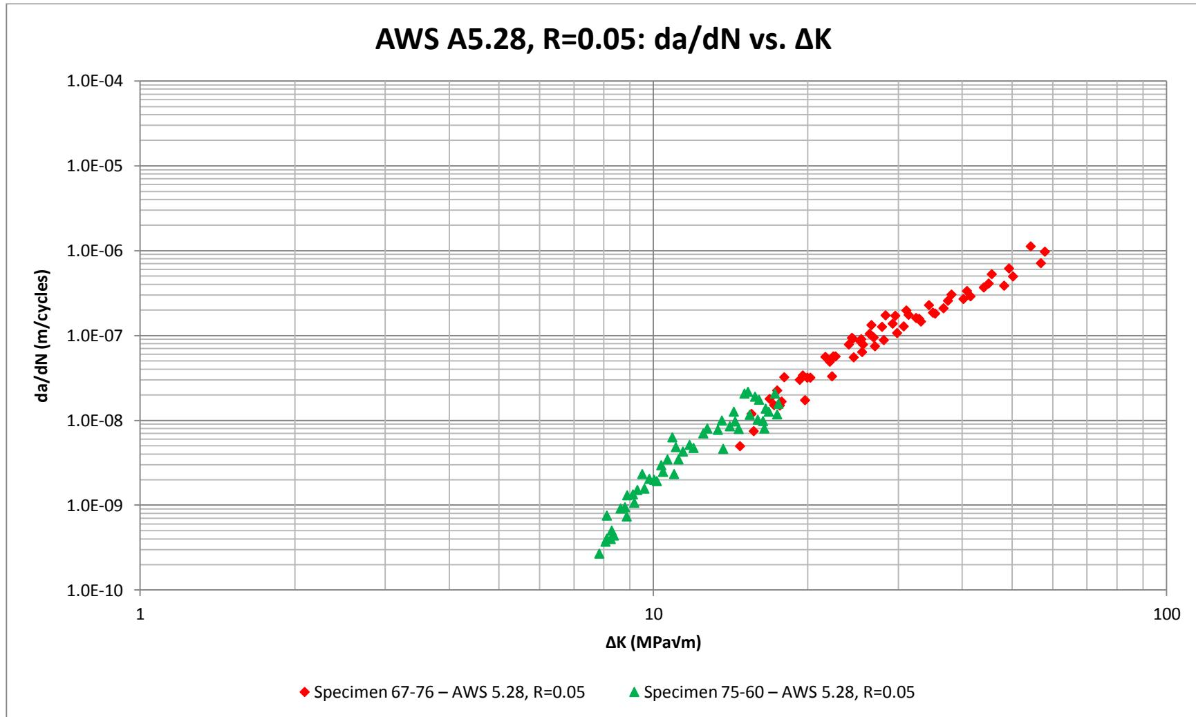
Figure H.10. Fatigue crack growth data for AWS A5.28 at stress ratio R=0.05 with a test frequency of 60Hz.
