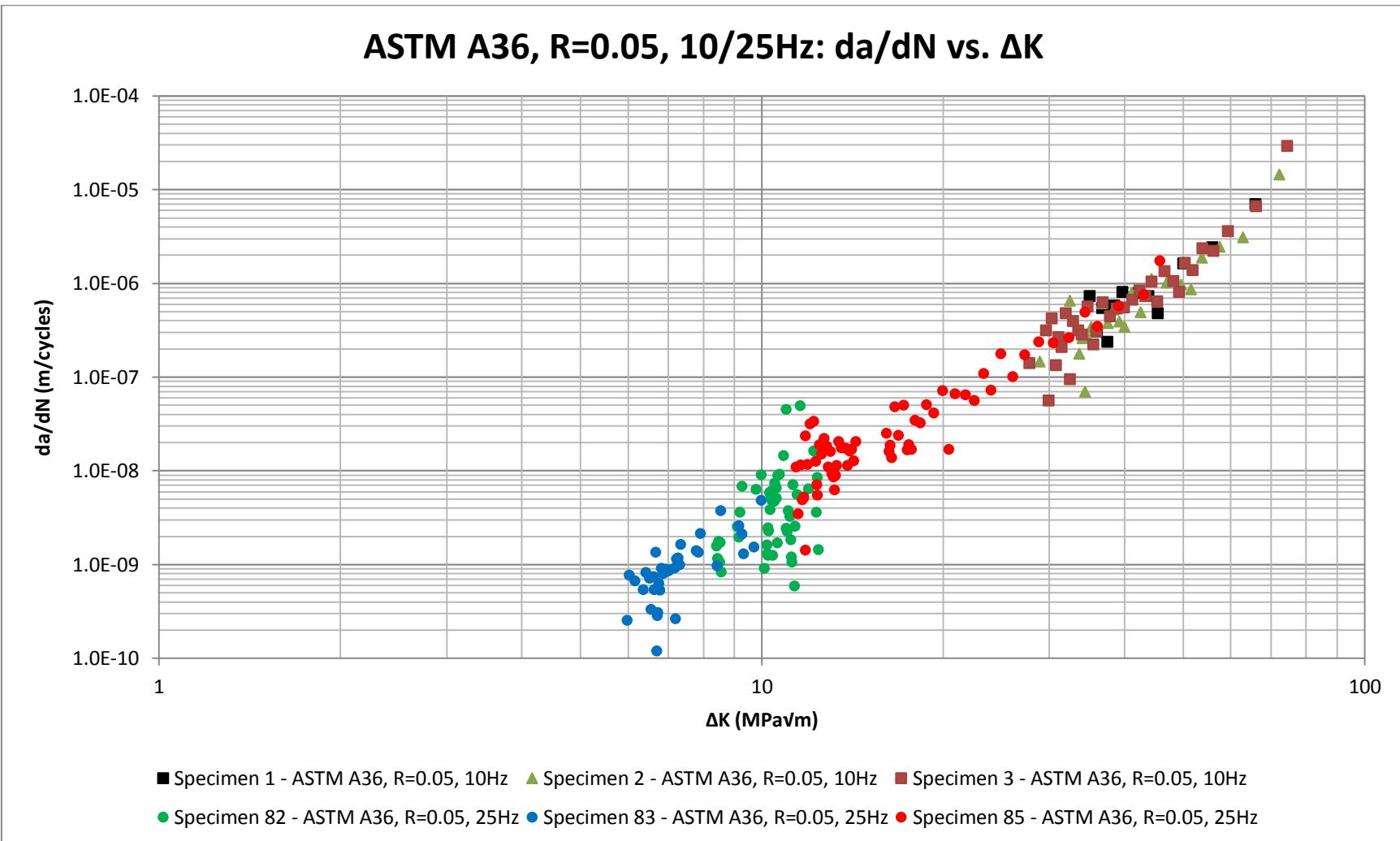
Figure H.1. Fatigue crack growth data for ASTM A36 at stress ratio R=0.05 with a test frequency of 25Hz and 10Hz.
