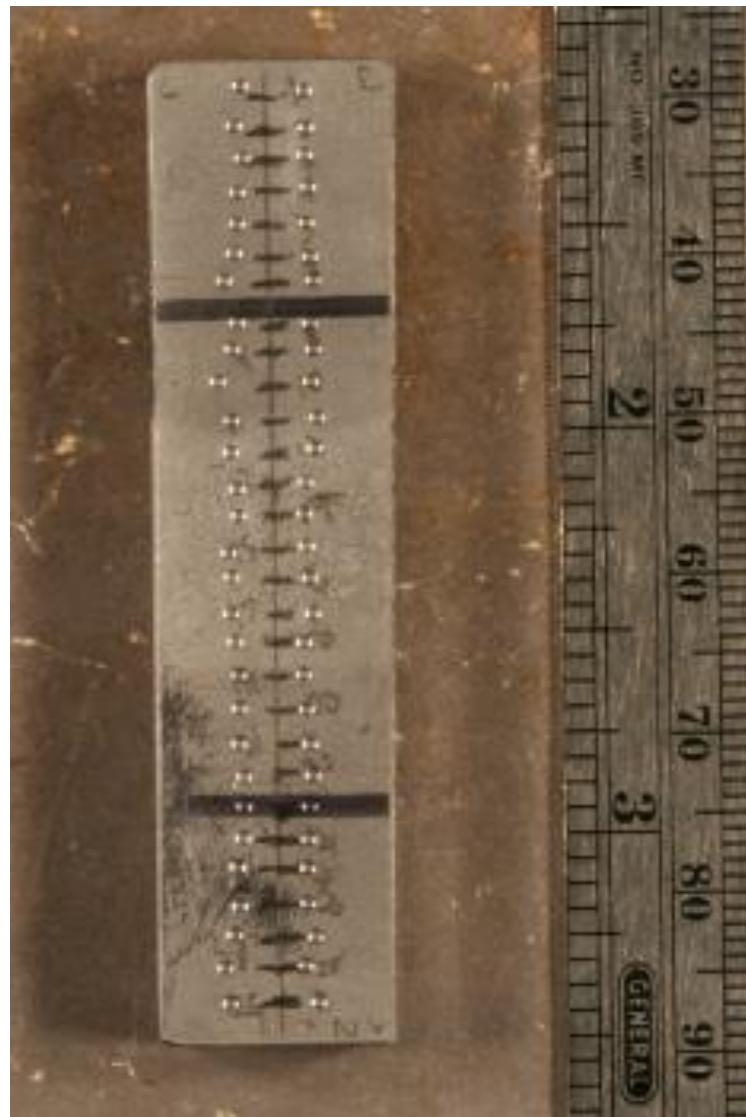
Figure E.1. Hardness gradient measurement profile on chemically etched test specimen - Specimen #37-31 AWS A5.18.
