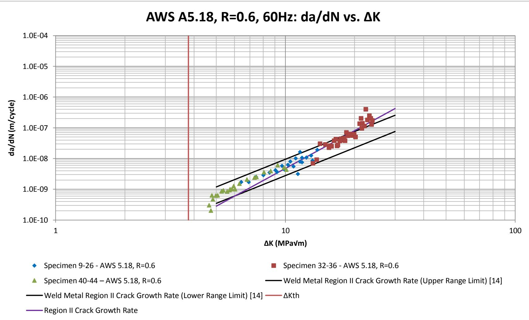
Figure 4.10. AWS A5.18 fatigue crack propagation results for  $R=0.6$ .
