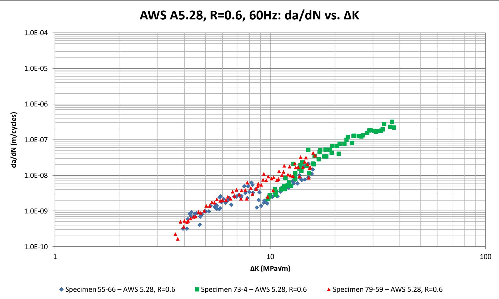
Figure H.12. Fatigue crack growth data for AWS A5.28 at stress ratio R=0.6 with a test frequency of 60Hz.
