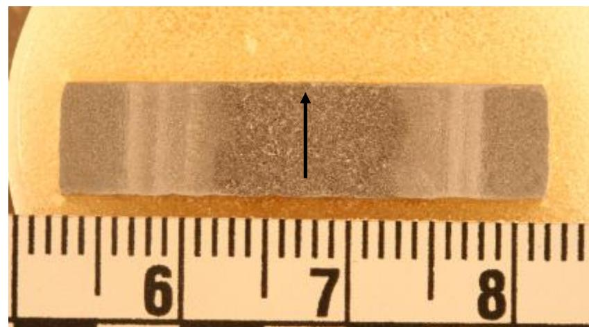
Figure D.8. AWS A5.18 metallographic specimen. Specimen was mounted in orientation where the crack would grow in the direction of the arrow.
