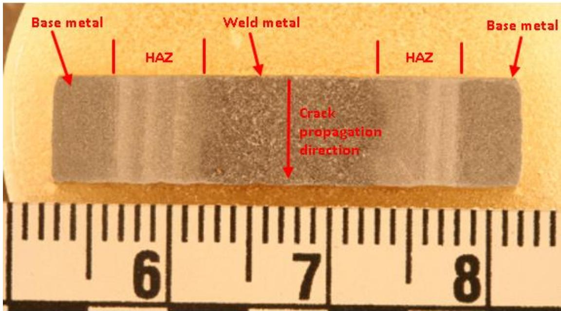
Figure 4.2. Macroscopic view of a polished and etched section of the weld zone cut from an AWS A5.18 weld fatigue specimen parallel to the surface of the specimen showing the 15 mm weld zone through which a crack propagates. HAZ = heat affected zone.
