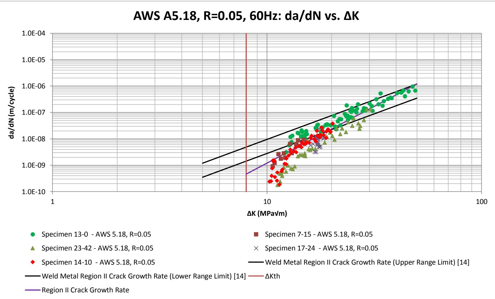
Figure 4.9. AWS A5.18 fatigue crack propagation results for  $R=0.05$ .
