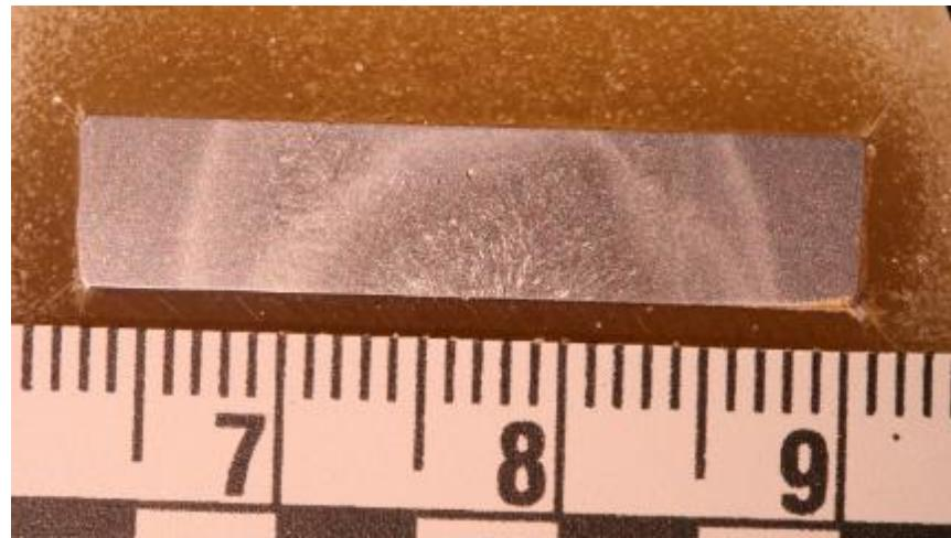
Figure D.7. AWS A5.18 metallographic specimen. Specimen was mounted in orientation for which the crack would grow perpendicular into the specimen.
