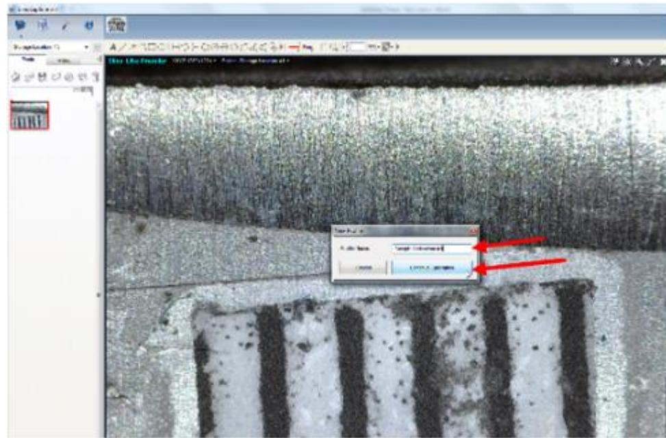
3. Press F8 or select Freeze. Enter the magnification of the camera (located on the side of the camera). Press enter when complete.
