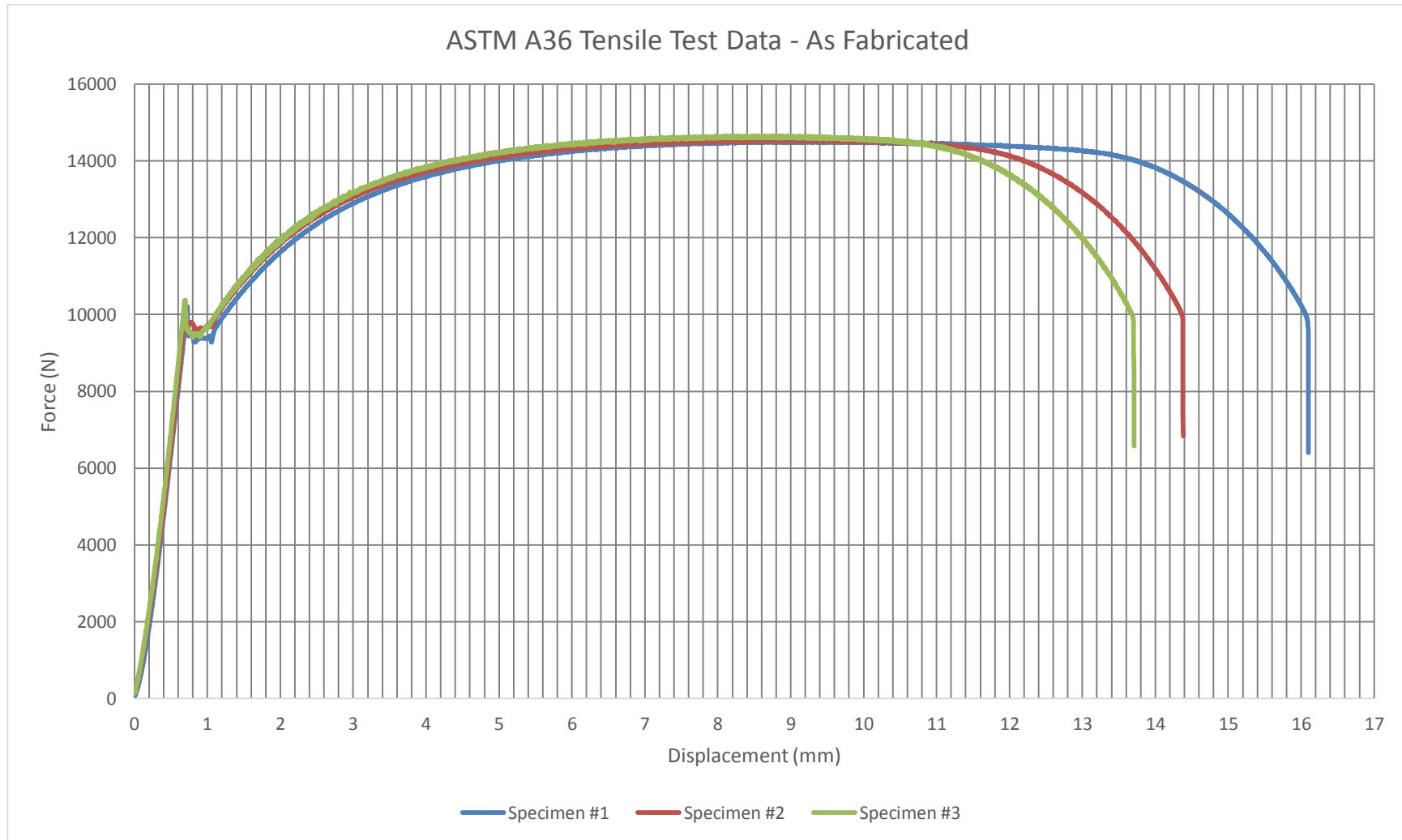
Figure C.1. Tensile test data from as fabricated tensile test specimens – ASTM A36
