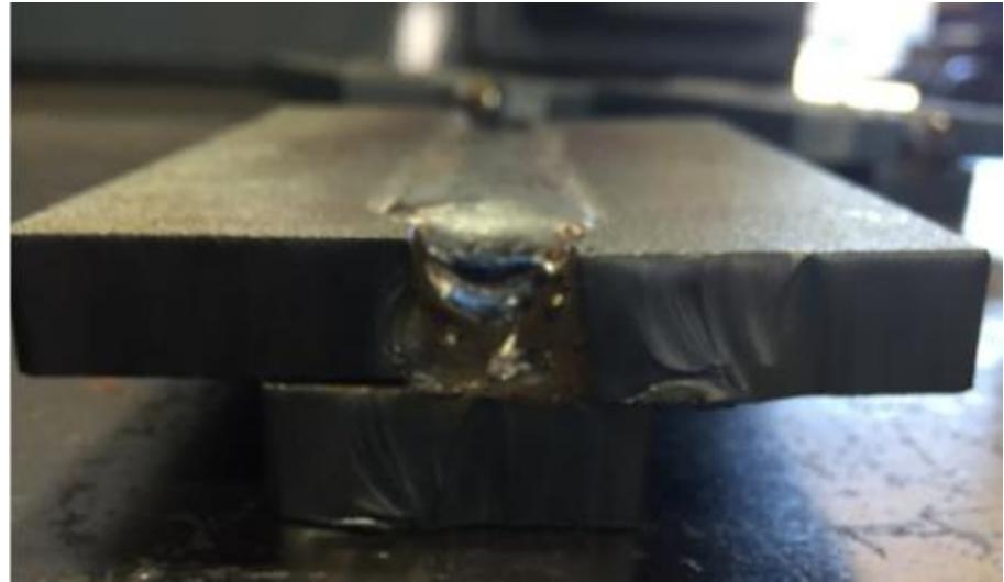
Figure 3.5. Specimen as welded (end view)
