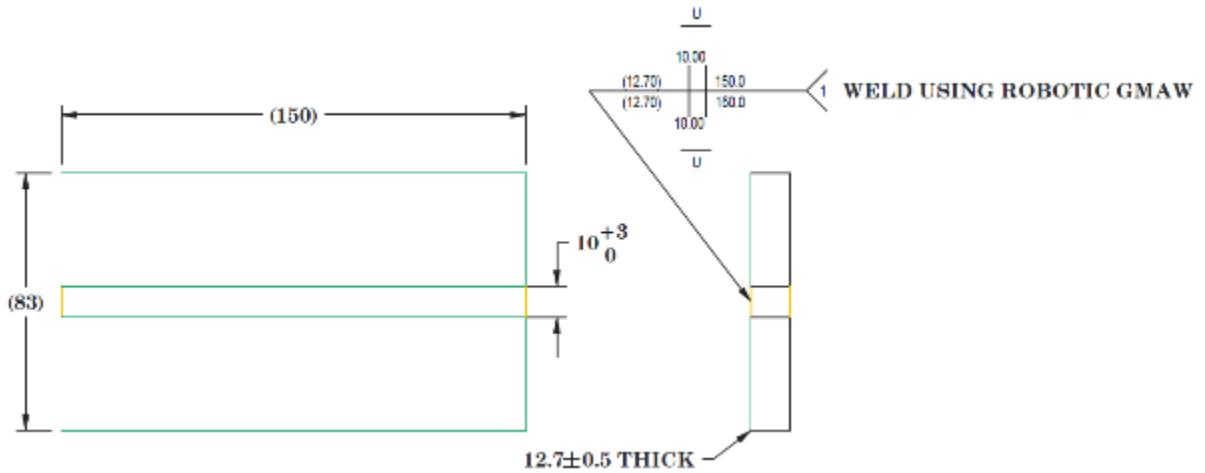
Figure 3.3. Welded specimen geometry after welding (units: mm)
