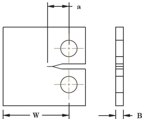
Figure 3.7. Compact C(T) specimen dimension used to calculate stress intensity range
