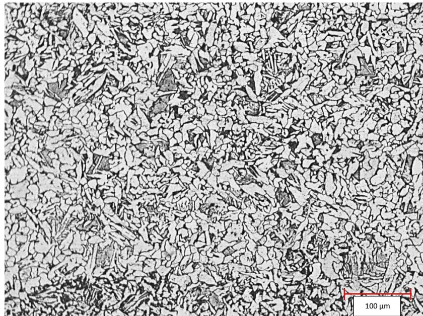
Figure 4.3. AWS A5.28 test specimen base metal microstructure. Microstructure is identical to base metal microstructure as shown in Figure 4.1.
