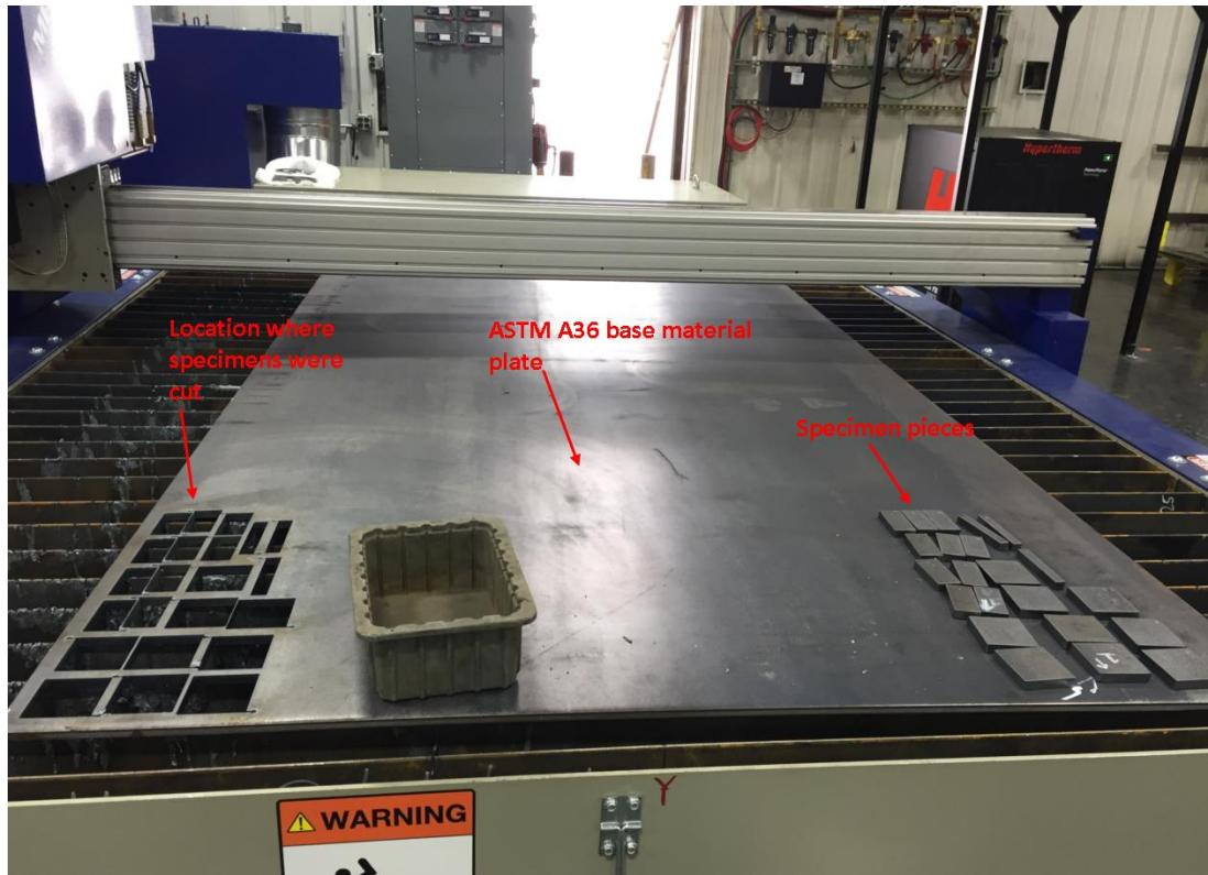
Figure 3.2. Specimen location and numbering on plasma cutter
