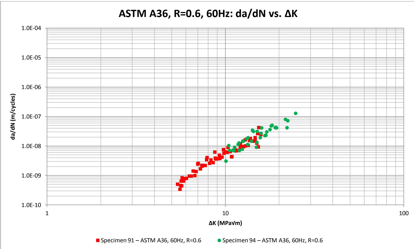
Figure H.3. Fatigue crack growth data for ASTM A36 at stress ratio R=0.6 with a test frequency of 60Hz.
