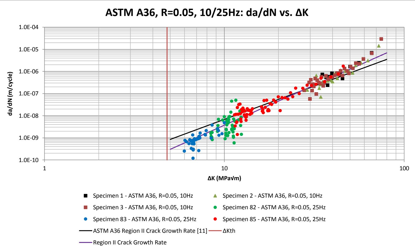
Figure 4.7. ASTM A36 fatigue crack propagation data for  $R=0.05$ .
