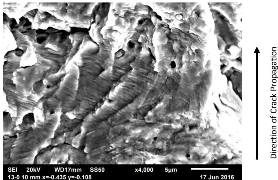
Figure 4.21. High magnification image of fracture surface for Specimen #13-0 - AWS A5.18 taken at  $a=22.6$  mm and showing well defined fatigue striations. Average striation spacing is 0.2  $\mu\text{m}$ .
