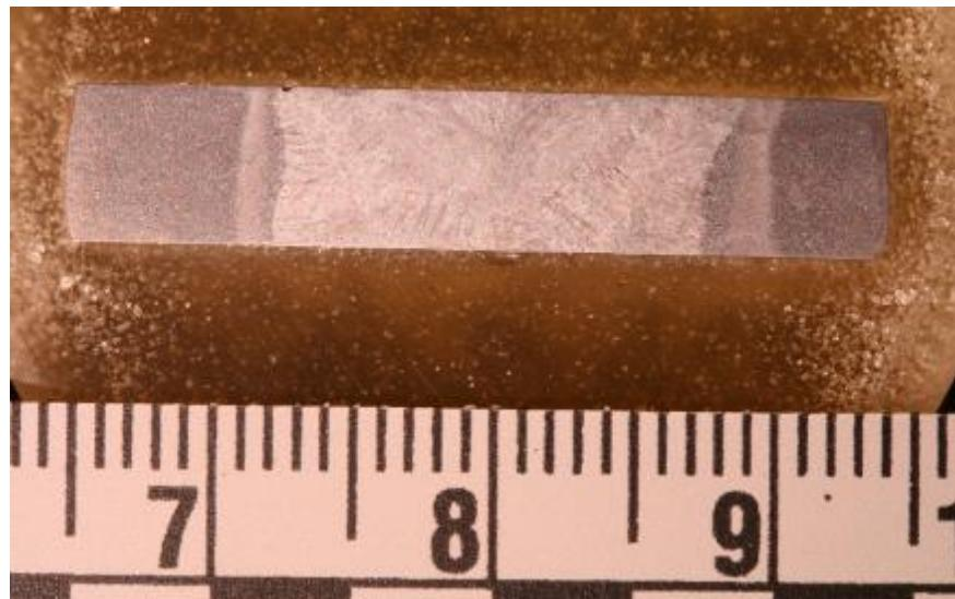
Figure D.5. AWS A5.28 metallographic specimen. Specimen was mounted in orientation for which the crack would grow perpendicular into the specimen.
