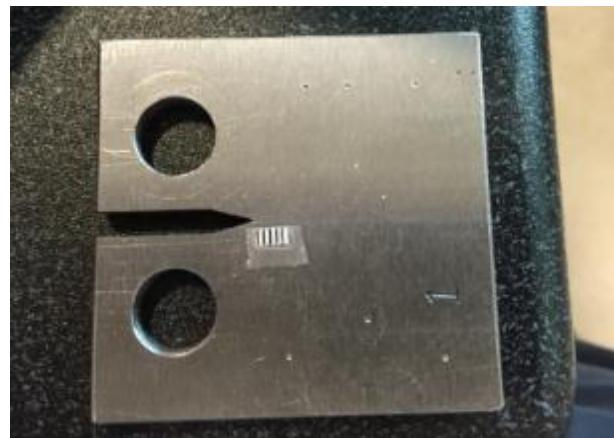
Figure 3.6. Finished compact C(T) specimen (after machining)
