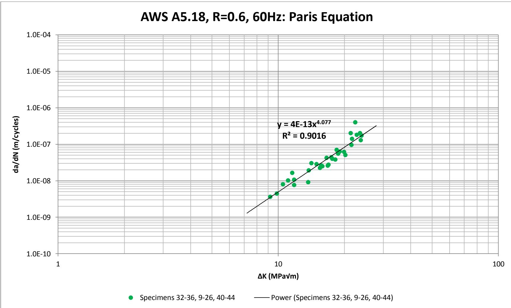
Figure H.9. Crack growth rate data and Paris Equation for AWS A5.18 at stress ratio R=0.6 with a test frequency of 60Hz.
