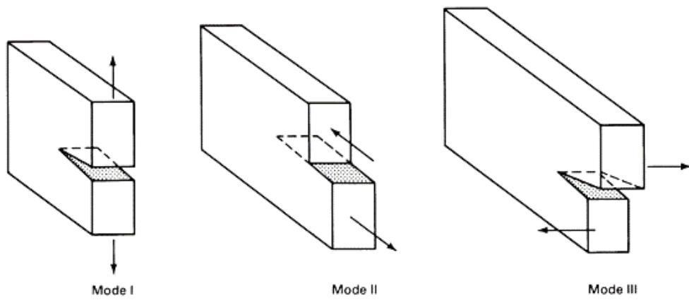
Figure 2.2. Three modes of loading that can be applied to a crack. [8]
