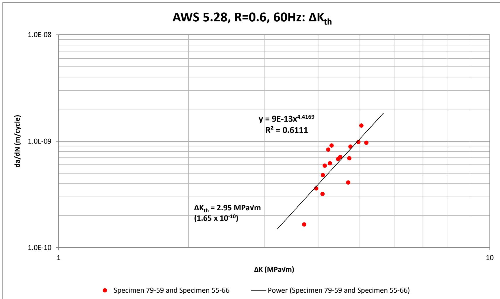
Figure 4.19.  $\Delta K_{th}$  data for AWS A5.28 at stress ratio R=0.6 with a test frequency of 60Hz.
