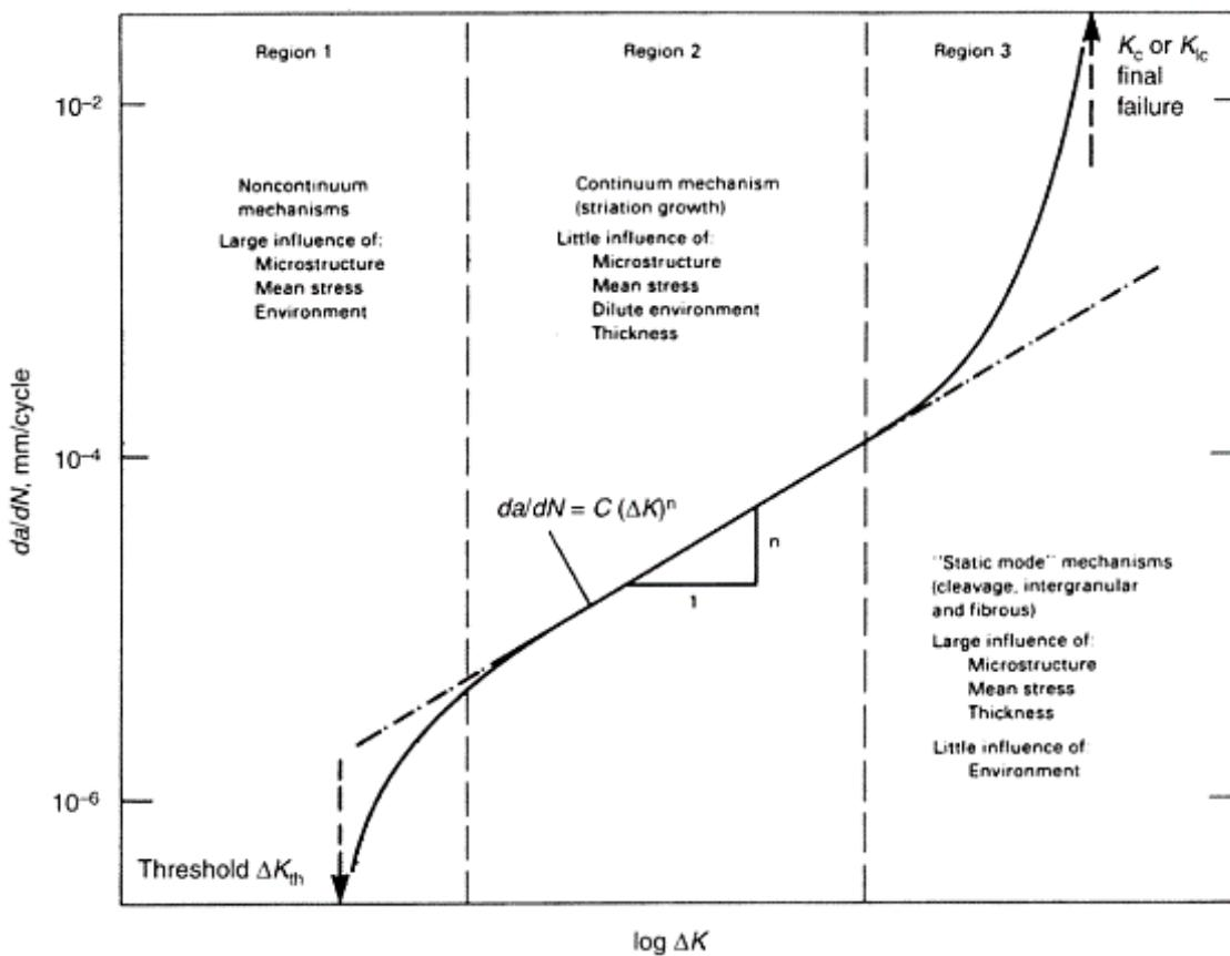
Figure 2.3.  $\log \frac{da}{dN}$  vs.  $\log \Delta K$  plot describing the three regions associated with crack growth rate. [5]
