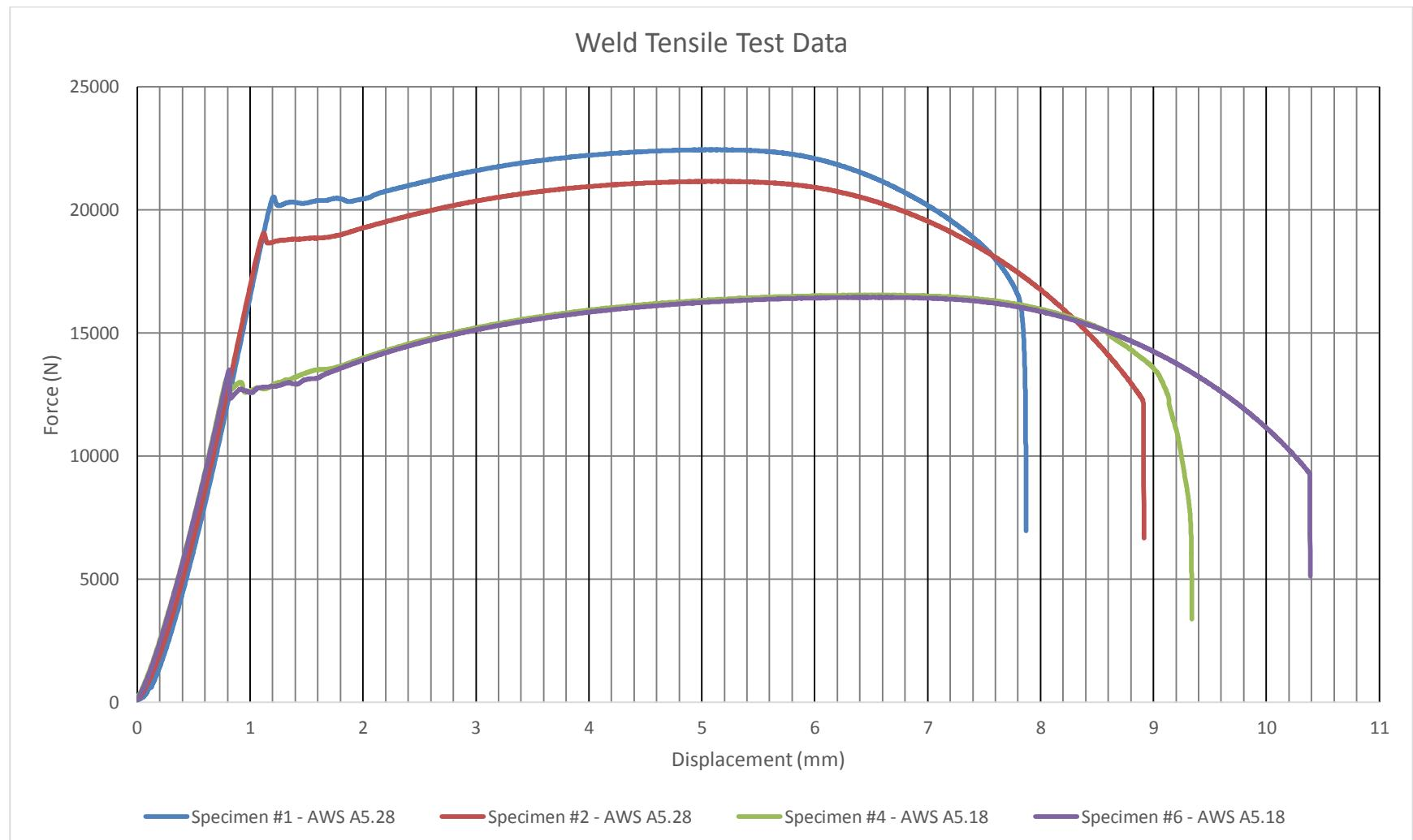
Figure C.4. Tensile test data for weld metal AWS A5.18 and AWS A5.28
