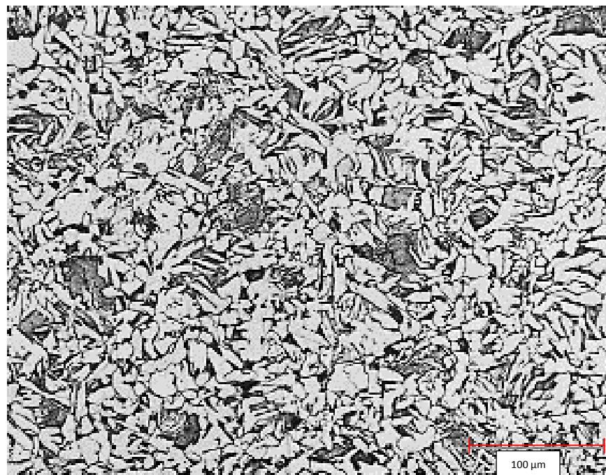
Figure 4.1. ASTM A36 base metal microstructure consisting of proeutectoid ferrite and pearlite.
