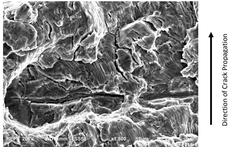
Figure 4.20. High magnification image of fracture surface for Specimen #3 – ASTM A36. Image taken at  $a=23.6$  mm and showing well defined fatigue striations and secondary cracks. Average striation spacing is 1.0  $\mu\text{m}$ .
