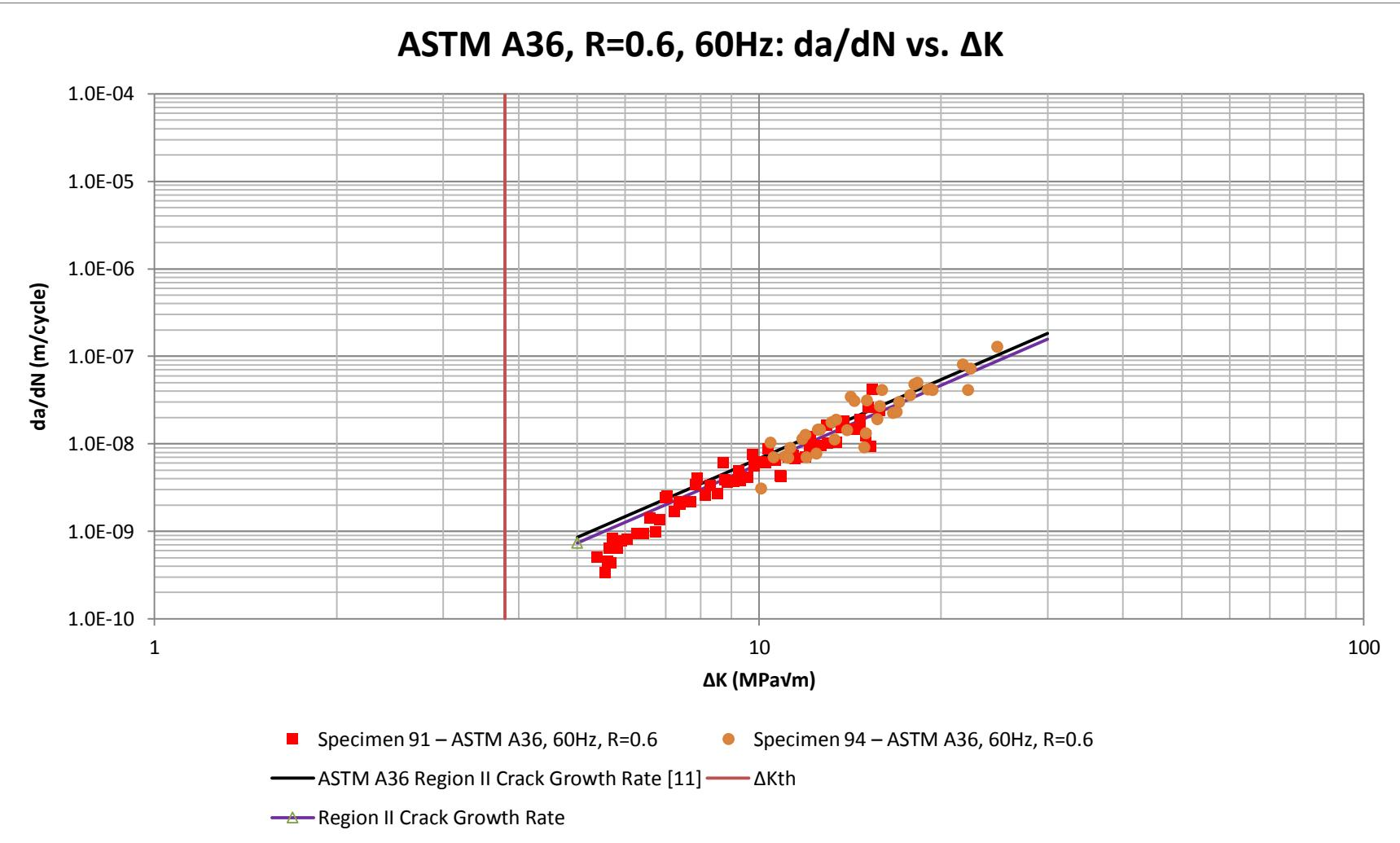
Figure 4.8. ASTM A36 fatigue crack propagation data for  $R=0.6$ .
