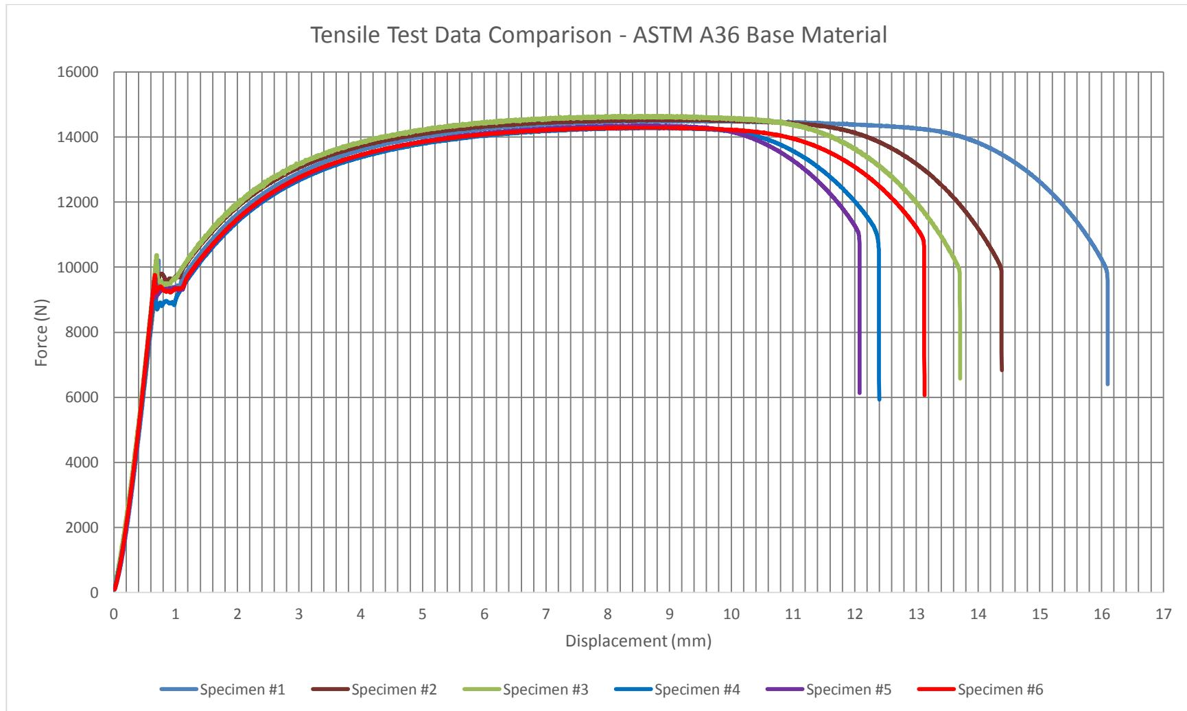
Figure C.3. Tensile test data comparison for ASTM A36 base material
