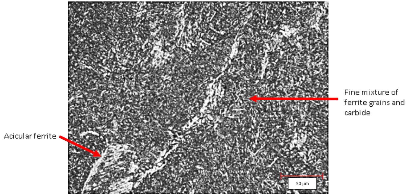
Figure 4.6. AWS A5.28 microstructure consisting of a fine mixture of ferrite grains and carbides as well as a small mixture of acicular ferrite.
