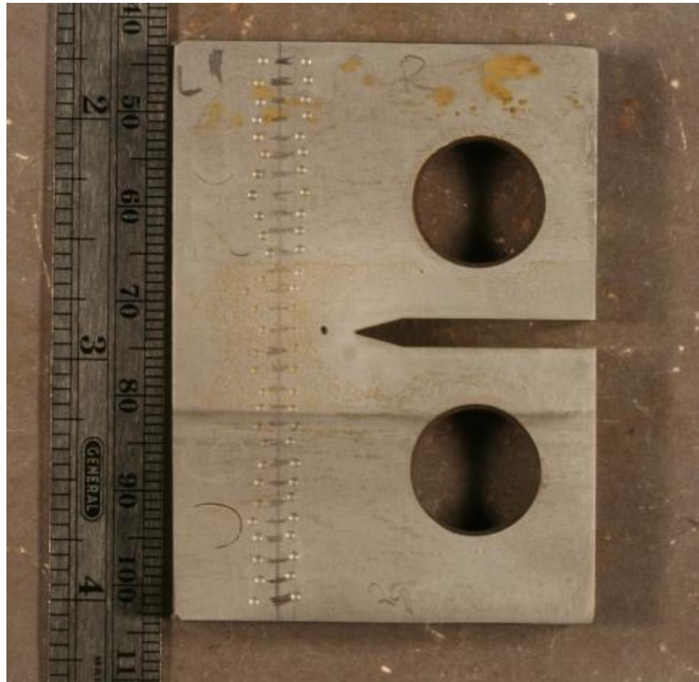
Figure E.2. Hardness gradient measurement profile on chemically etched test specimen - Specimen #52-90 AWS A5.28.
