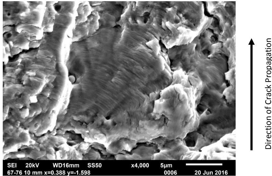
Figure 4.22. High magnification image of fracture surface for Specimen #67-76 - AWS A5.28 taken at  $a=22.5$  mm and showing well defined fatigue striations. Average striation spacing is  $0.18 \mu\text{m}$ .
