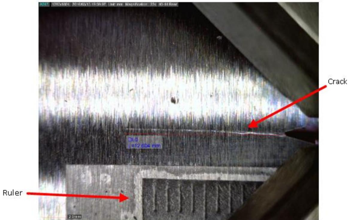
Figure 3.8. Crack measurement photo showing crack and calibration ruler in mm.
