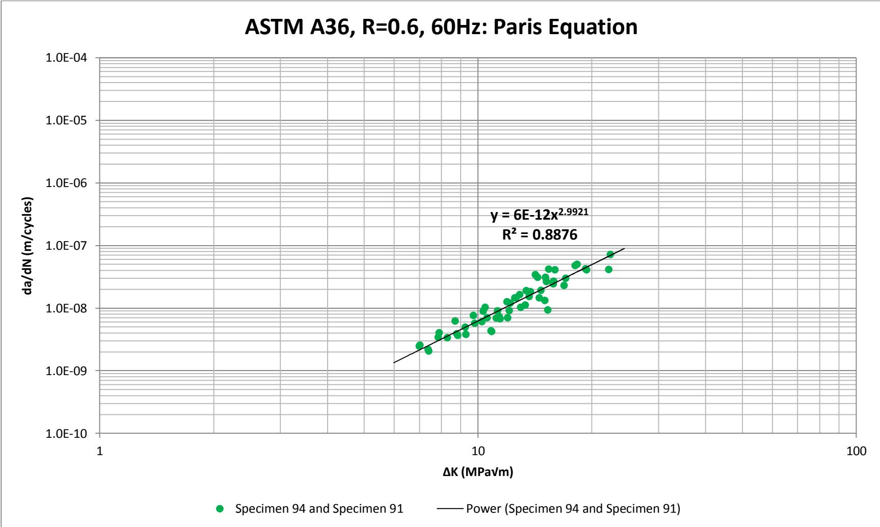
Figure H.4. Fatigue crack growth data and Paris Equation for ASTM A36 at stress ratio R=0.6 with a test frequency of 60Hz.
