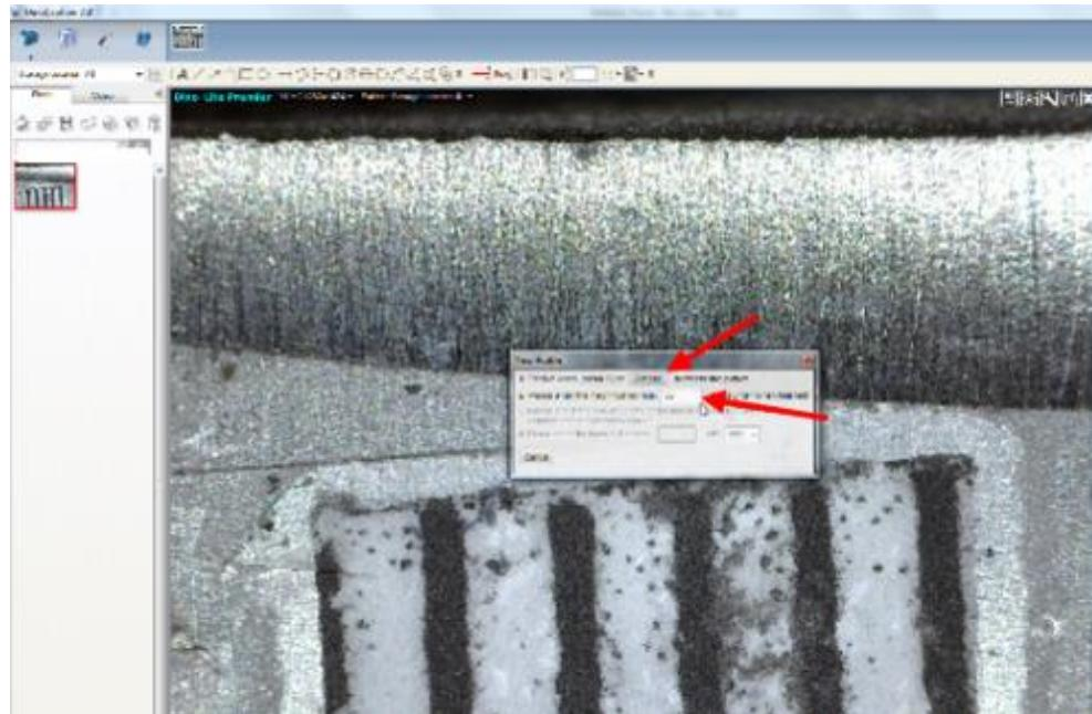
4. Align the H-frame around the ruler. Make the H-frame as wide as possible and utilize the ends of each mark for a precise calibration. To move the H-frame click the small box where the vertical and horizontal lines intersect. To place click on desired location.
