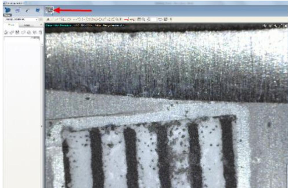
2. Microscope is now viewable. Adjust camera magnification and position until the desired picture is achieved. Select camera icon to take snapshot. Note: if measurement value is desired on picture it is most efficient to perform calibration and add measurement before taking picture. The measurement can always be added after the picture has been taken.
