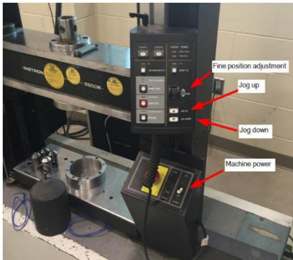
Figure B.1. Instron machine system controls
