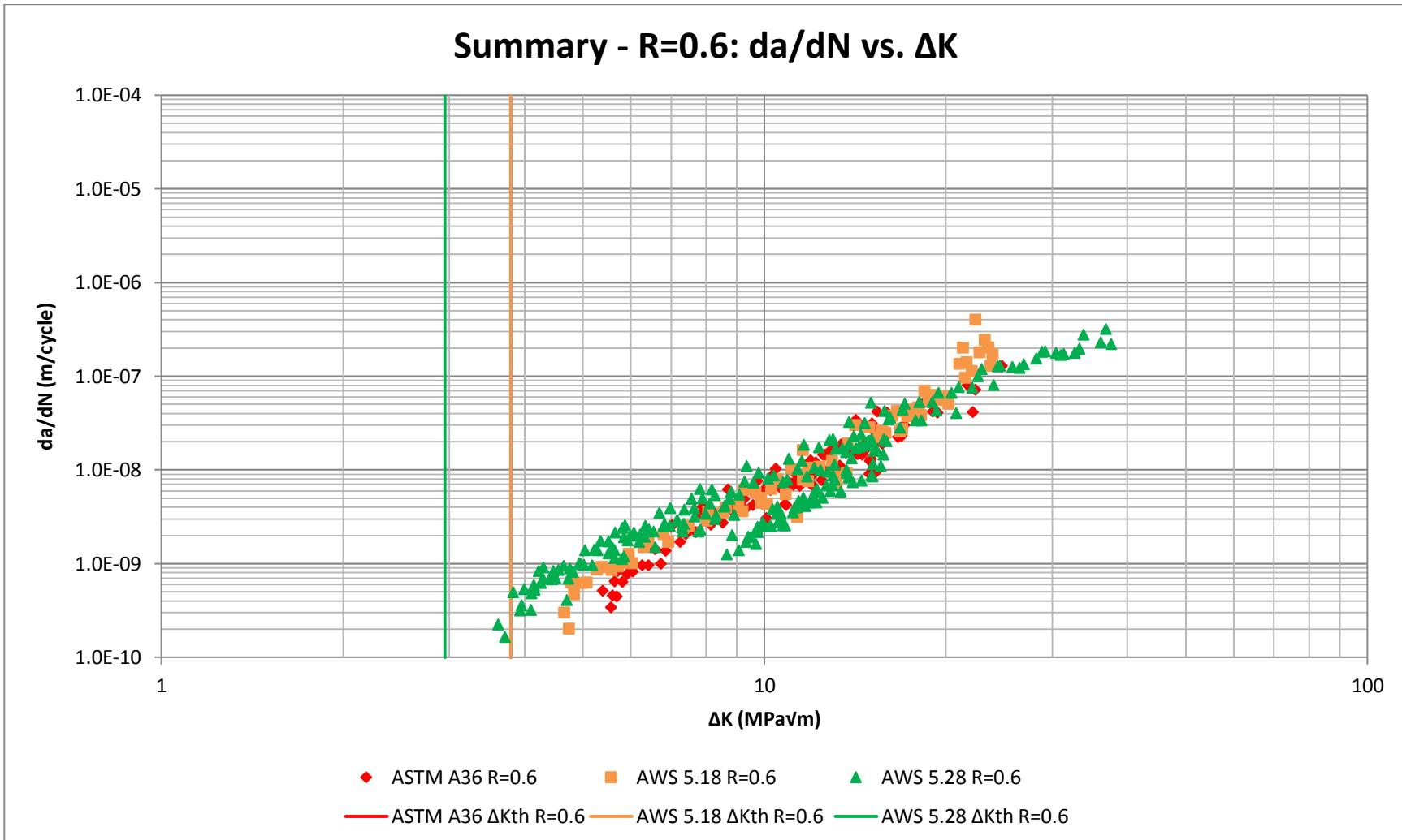
Figure 5.2. Summary of all fatigue crack propagation results for  $R=0.6$ .  $\Delta K_{th}=3.80$  for both ASTM A36 and AWS A5.18.
