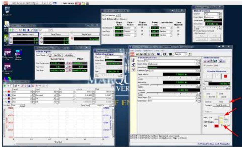
11. Move the Manual Command Slider bar until the Axial Force value (listed in Station Signals) reads 0 lb<sub>f</sub>.
