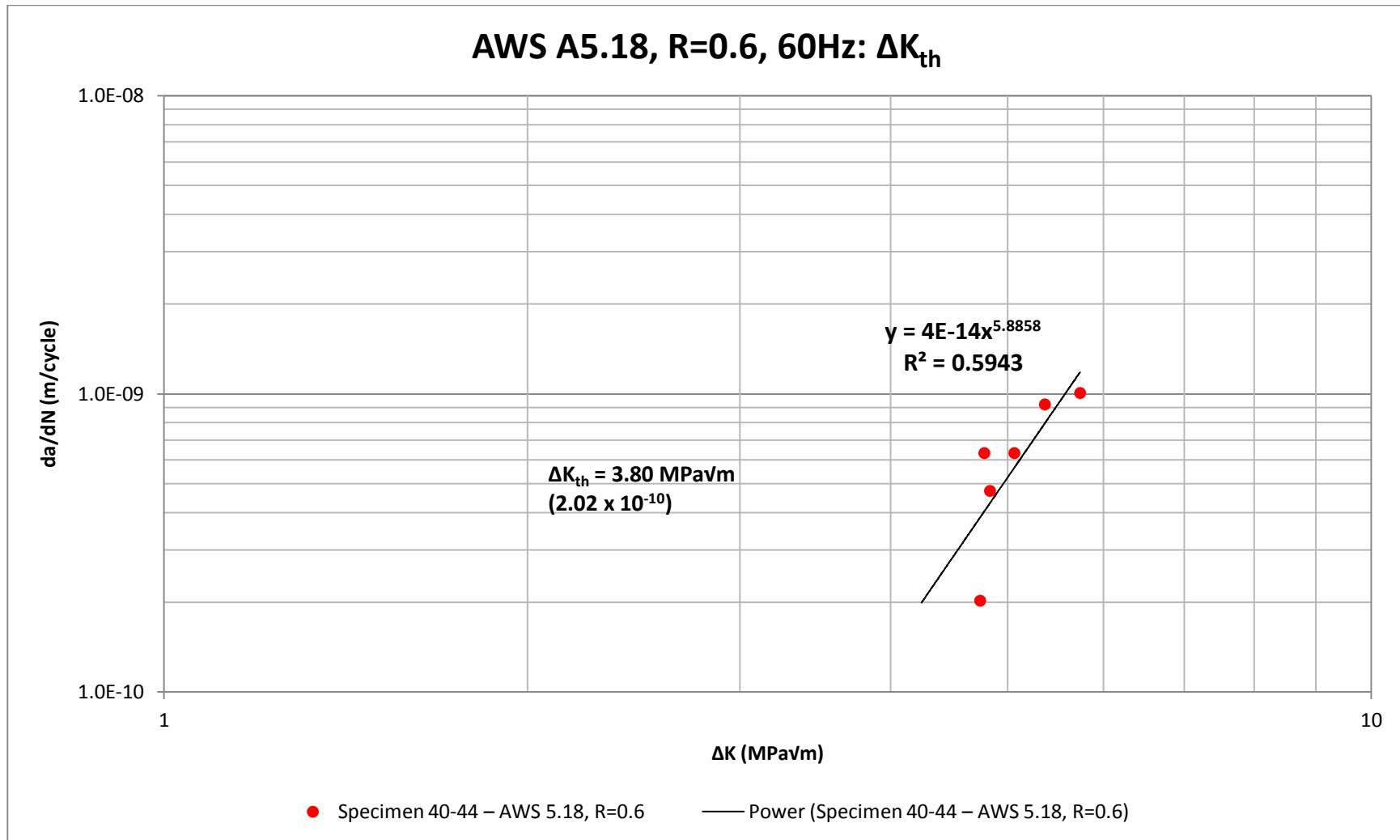
Figure 4.17:  $\Delta K_{th}$  data for AWS A5.18 at stress ratio R=0.6 with a test frequency of 60Hz.
