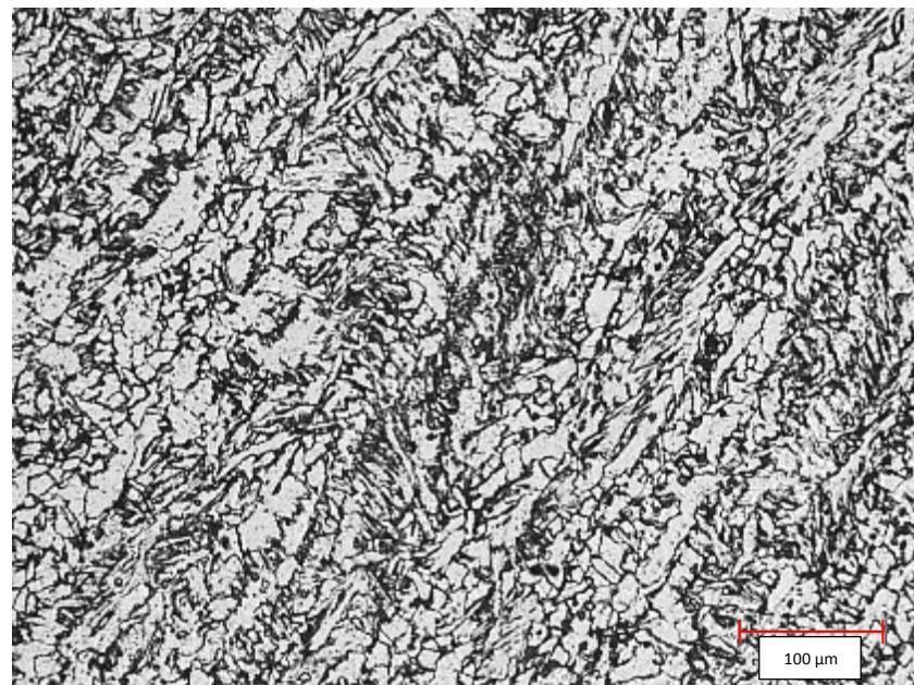
Figure 4.4. AWS A5.18 microstructure consisting of acicular ferrite and carbides.
