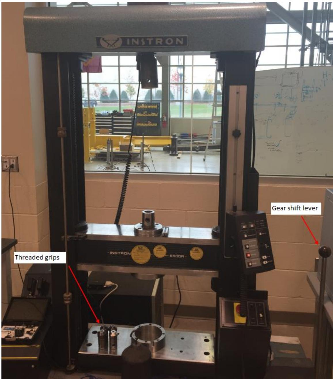
Figure B.3. Grip and gear shift lever identification
