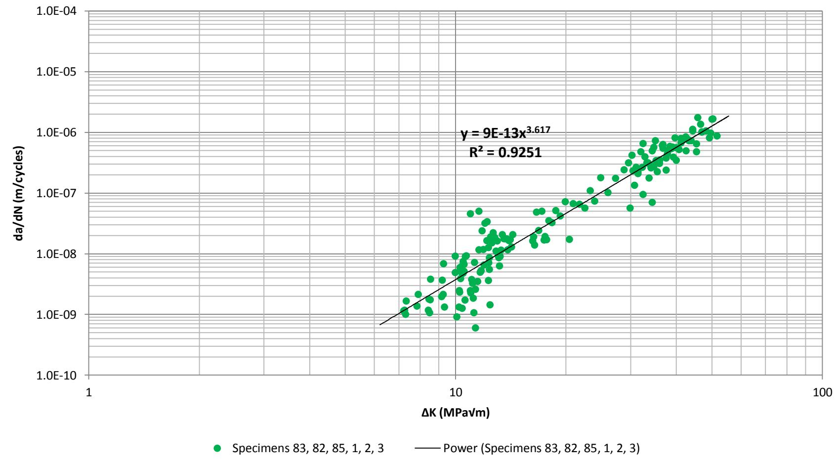
Figure H.2. Crack growth rate data and Paris Equation for ASTM A36 at stress ratio R=0.05 with a test frequency of 10 and 25Hz.
