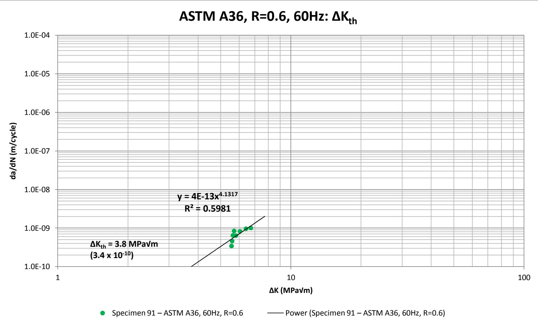
Figure 4.15.  $\Delta K_{th}$  data for ASTM A36 at stress ratio R=0.6 with a test frequency of 60Hz.
