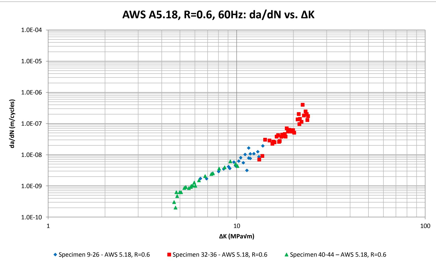
Figure H.8. Fatigue crack growth data for AWS A5.18 at stress ratio  $R=0.6$  with a test frequency of 60Hz.
