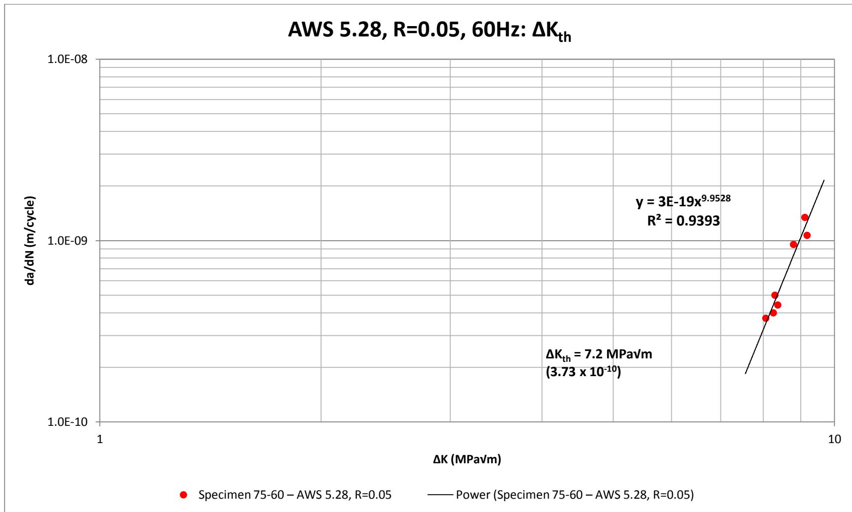
Figure 4.18.  $\Delta K_{th}$  data for AWS A5.28 at stress ratio R=0.05 with a test frequency of 60Hz.
