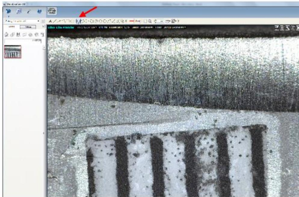
8. Select two point to measure. Click on the first position and click on the second position to complete the measurement.
