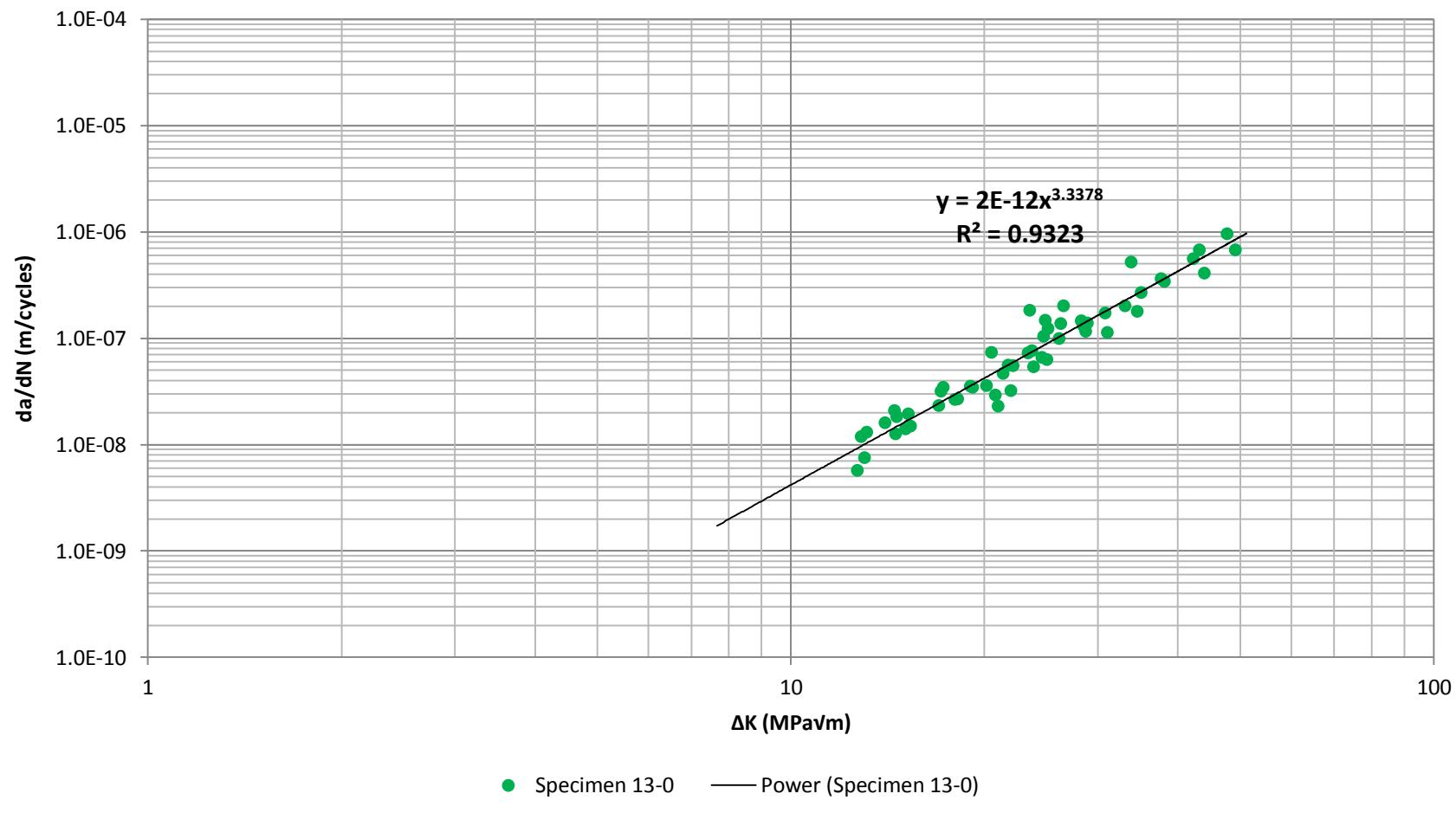
Figure H.7. Paris Equation for Specimen 13-0 AWS A5.18 at stress ratio  $R=0.6$  with a test frequency of 60Hz.
