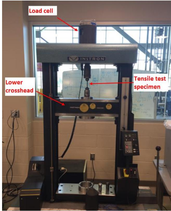
Figure 3.9. Instron Tensile Test Machine
