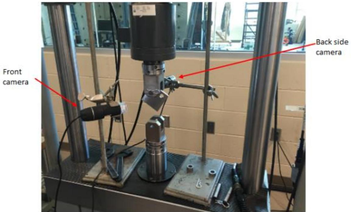
17. Move the lower grip into a position where it is possible to install the lower grip pin. The lower grip is moved with the Manual Control slide bar. Ensure that specimen remains clear of lower grip as it approached the upper grip.
