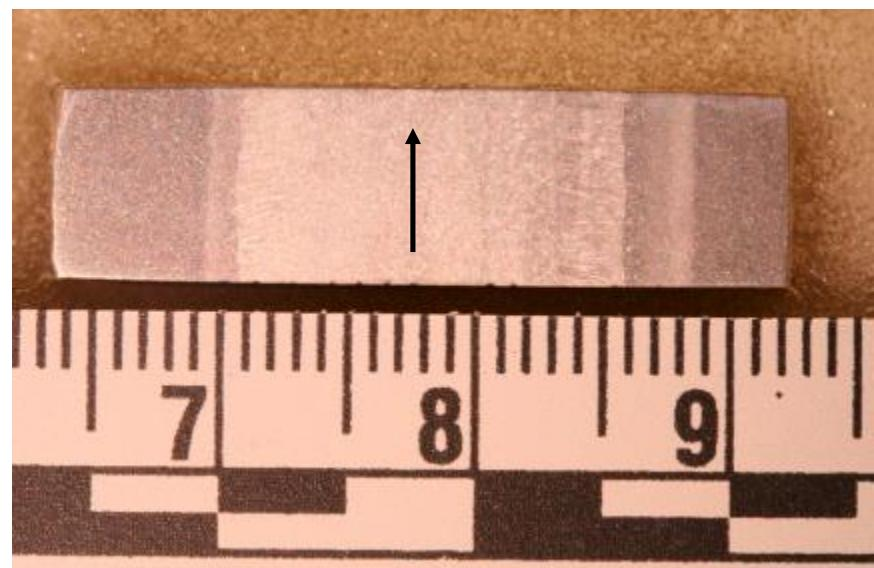
Figure D.6. AWS A5.28 metallographic specimen. Specimen was mounted in orientation for which the crack would grow in the direction of the arrow.
