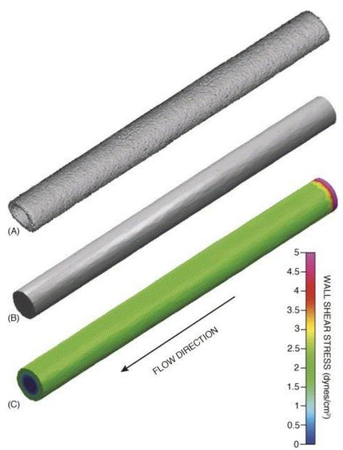
**Fig. 8.** Surface smoothing of a reconstructed polyethylene tube. Illustrations of a rendered polyethylene tube obtained before (A) and after (B) implementation of the surface smoothing operations discussed in the text. The uniformity of WSS distributions along the wall of the reconstructed and smoothed polyethylene tube is depicted in (C).
