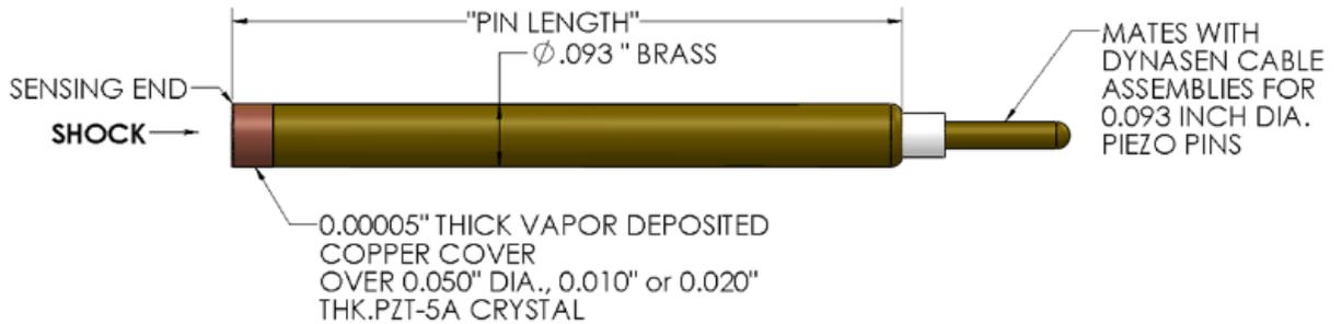
Figure 53: Piezoelectric Pin [19]
