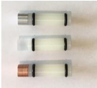
*Figure 29: Nylon sabots with two O-Rings and flyers inserted*
