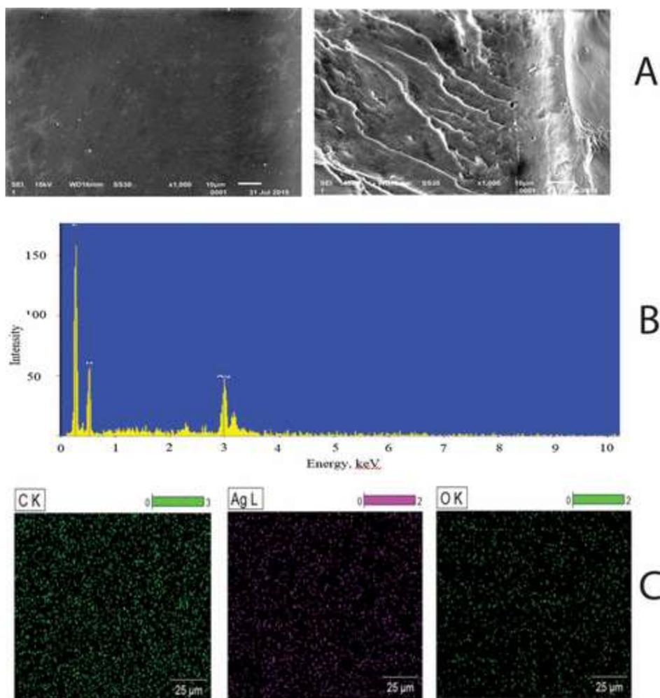
**Figure 3.** (A) SEM images of the [CEL+KER+AgNPs] composite: (left) surface image; (right) cross-sectional image. (B) EDS spectrum and (C) EDS images recorded for carbon (left), silver (middle), and oxygen (right) of the [CEL+KER+AgNPs] composite.
