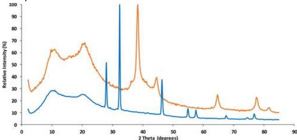
**Figure 2.** Powder XRD spectra of the [CEL+KER+Ag<sup>+</sup>NPs] (blue) and [CEL+KER+Ag<sup>0</sup>NPs] (orange) composites.
