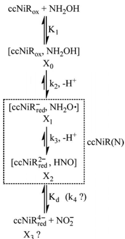
Scheme 3. Minimal Model for the Interaction of Hydroxylamine with ccNiR<sub>ox</sub> That Considers Kinetic and Thermodynamic Observations<sup>a</sup>
