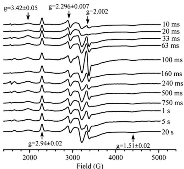
Figure 5. Results of the rapid-freeze-quench experiments. Changes observed in the X-band EPR spectrum of ccNiR at various times after rapid mixing of 50  $\mu\text{M}$  resting enzyme with 200 mM hydroxylamine. All data were collected in perpendicular mode, at 9.39 GHz. Signals were normalized to the peak at 2290 G.
