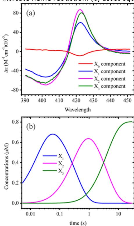
Figure 2. (a) Extinction coefficient difference spectra of spectral components  $X_0$ – $X_3$  (Scheme 1), calculated by fitting the data depicted in Figure 1 with a three-exponential function and four spectral components. The  $\lambda_{\text{max}}$  of the reduced heme peak at 424 nm increases in amplitude from the first intermediate to the second and then
