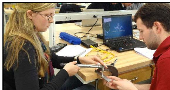
Figure 8: Measuring bolt clamping force in Experiment 7.
