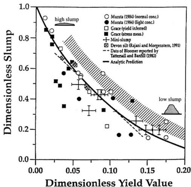
Fig. 2—Plot for estimating yield stress value from slump data.<sup>15</sup>
