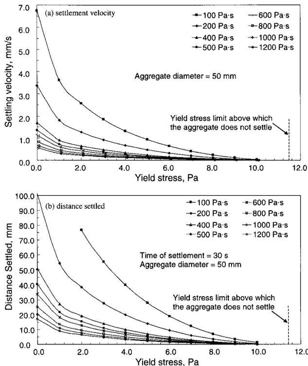
Fig. 5—Settling velocity (a), and distance settled in 30 s (b) of 50 mm coarse aggregate in mortar for different values of Bingham yield stress and plastic viscosity.
