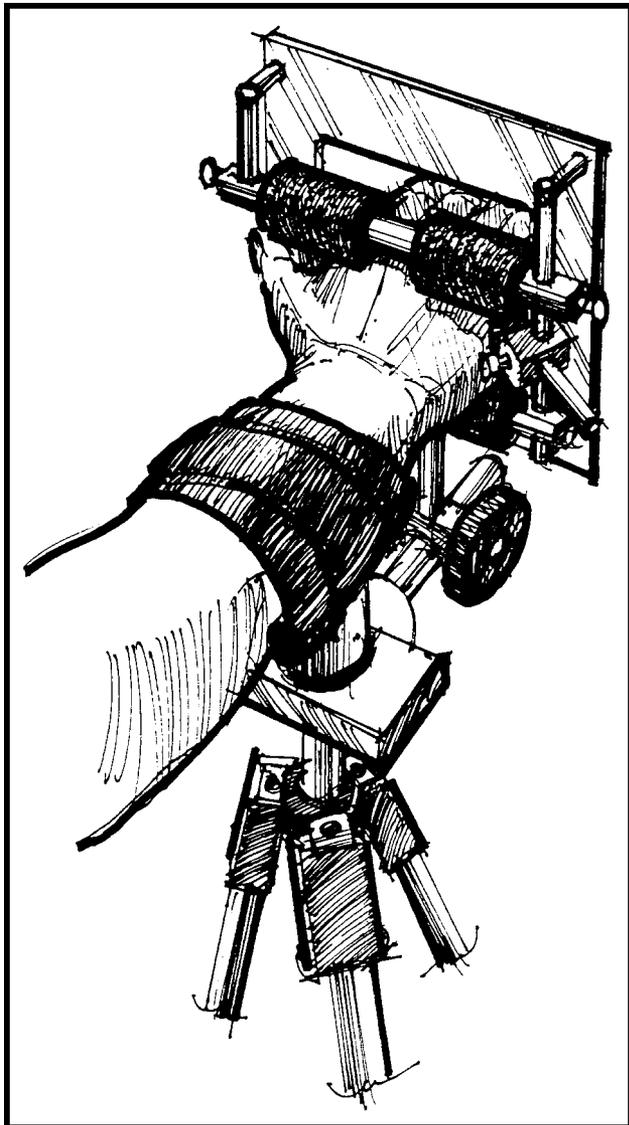
**Figure 5.** Custom-built fixture to allow subjects to make maximum voluntary contractions (MVCs) so that maximal electromyographic voltages (100% MVC) of the extensor carpi ulnaris, flexor carpi ulnaris, and flexor carpi radialis muscles could be monitored.
