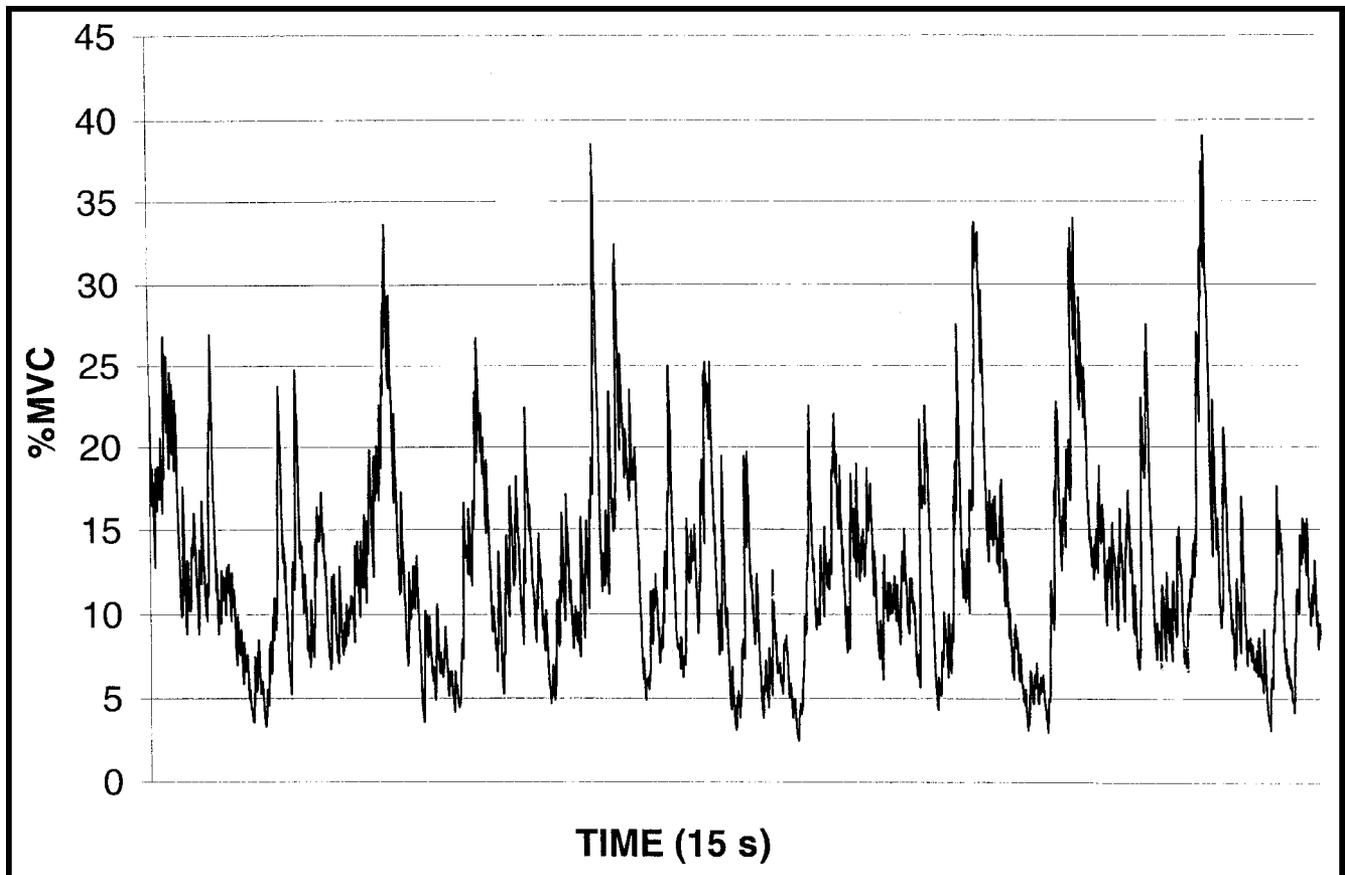
**Figure 4.** Fifteen seconds of normalized root-mean-square electromyographic data of the right extensor carpi ulnaris muscle expressed as a percentage of maximum voluntary contraction. The keyboard was at a positive slope of 7.5 degrees.
