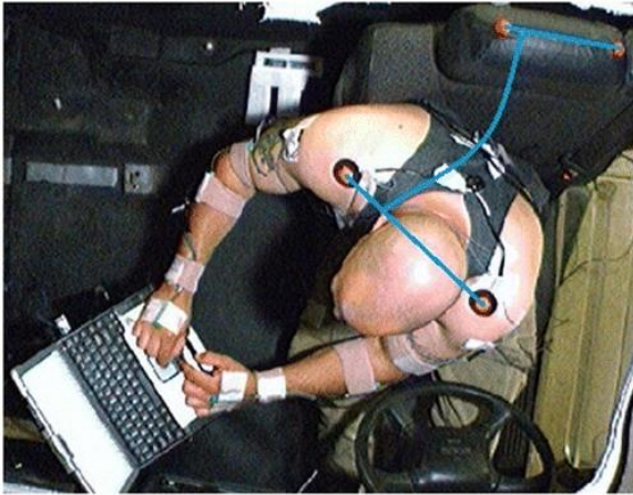
Figure 5. Markers located on the participant's acromions. Lines were added post hoc in the photo to indicate the angle of shoulders to seat back.
