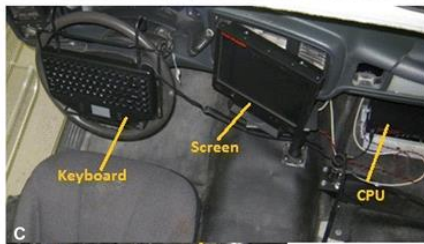
Figure 2. Laptop mount components and Hub Data911 M6 mounted in test cab.
