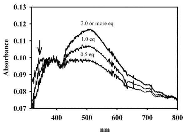
Figure 5 Spectrophotometric titration of apo-CcrA with Co(II). Apo-CcrA (360  $\mu$ M) in 50 mM Hepes, pH 7.6, was titrated with 0.5, 1.0, and 2.0 equiv of Co(II). The spectrum of apo-CcrA was subtracted from the spectra of the Co(II)-added enzymes.
