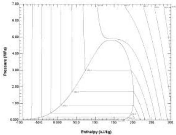
**Figure 2:** Pressure versus enthalpy diagram for R-23 (NIST 2007).
