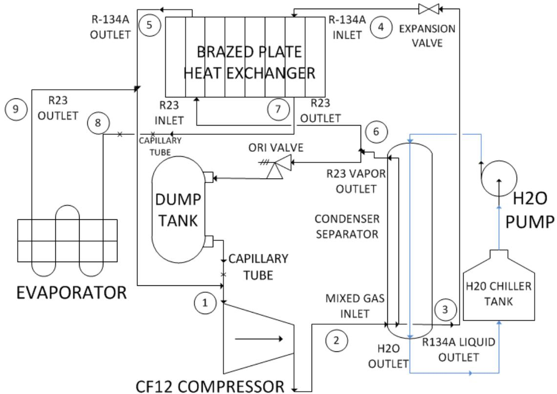
Figure 4: Mixed refrigerant test stand diagram.
