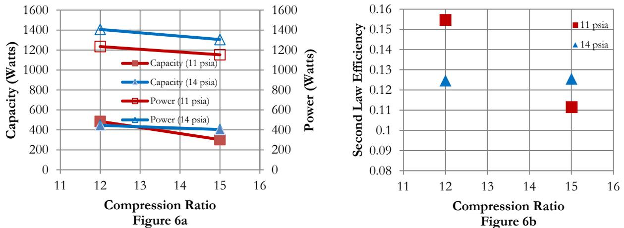
**Figure 6:** (a) Capacity and power consumption for suction pressure of 11 psia and 14 psia at varying compression ratios and (b) second law efficiency at suction pressures for varying compression ratios.
