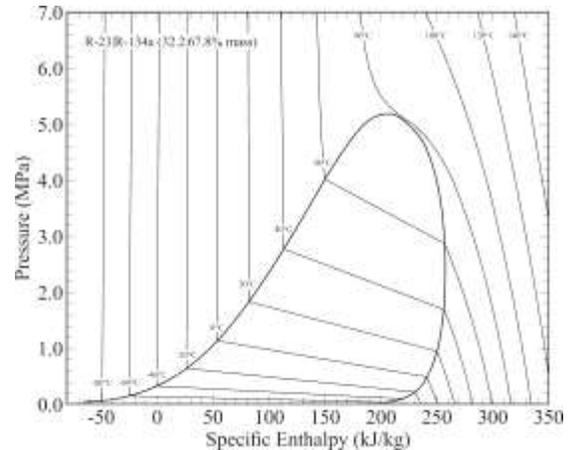
**Figure 3:** Pressure versus enthalpy diagram for R-23/R-134a refrigerant mixture (NIST 2007).
