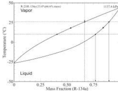
**Figure 5:** Binary phase diagram for 33.4% R-23 and 66.6% R-134a by mass at 1137.6 kPa (165 psia) (NIST 2007).
