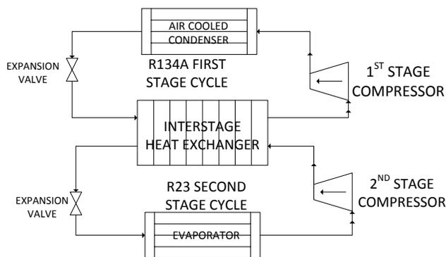
**Figure 1:** Two-stage cascade refrigeration system diagram.
