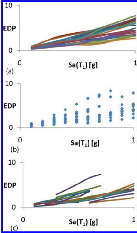
Figure 2. (a) Incremental dynamic analysis (IDA); (b) multiple stripe analysis (MSA); (c) adaptive incremental dynamic analysis (AIDA).
