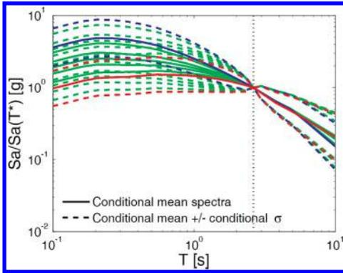
Figure 5. Normalized target response spectra conditional on  $Sa(2.6s)$ , to illustrate the change of spectral shape across IM levels. The lower-bound IM level (IM 1) corresponds to 50% in 30 years probability of exceedance, and the upper-bound IM level (IM 7) corresponds to 1% in 50 years probability of exceedance.
