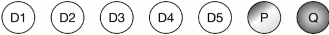
Fig. 1. A small reed-solomon linear code as used in a RAID level 6 stripe.
