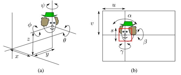
Figure 1: 6-DOF face pose representation in the world coordinates and in the image space. (a) 6-DOF pose in the world coordinates,  $\tilde{\mathbf{p}}_w = [x, y, z, \theta, \phi, \psi]^T$ . (b) 6-DOF pose in the image space,  $\tilde{\mathbf{p}}_i = [u, v, s, \alpha, \beta, \gamma]^T$ .
