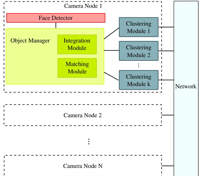
Figure 7: Block diagram of our distributed face tracker.
