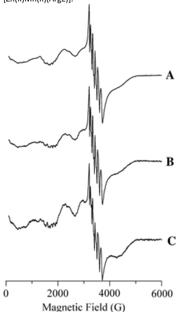
Fig. 10. EPR spectra of [\text{Mn(II)Mn(II)(ArgE)}] (A), [\text{Mn(II)Zn(II)(ArgE)}] (B), and [\text{Zn(II)Mn(II)(ArgE)}] (C) after incubation with bestatin in 50 mM HEPES buffer, pH 7.5. Spectra were recorded at 9.63 GHz, 12 K, 20-mW microwave power
