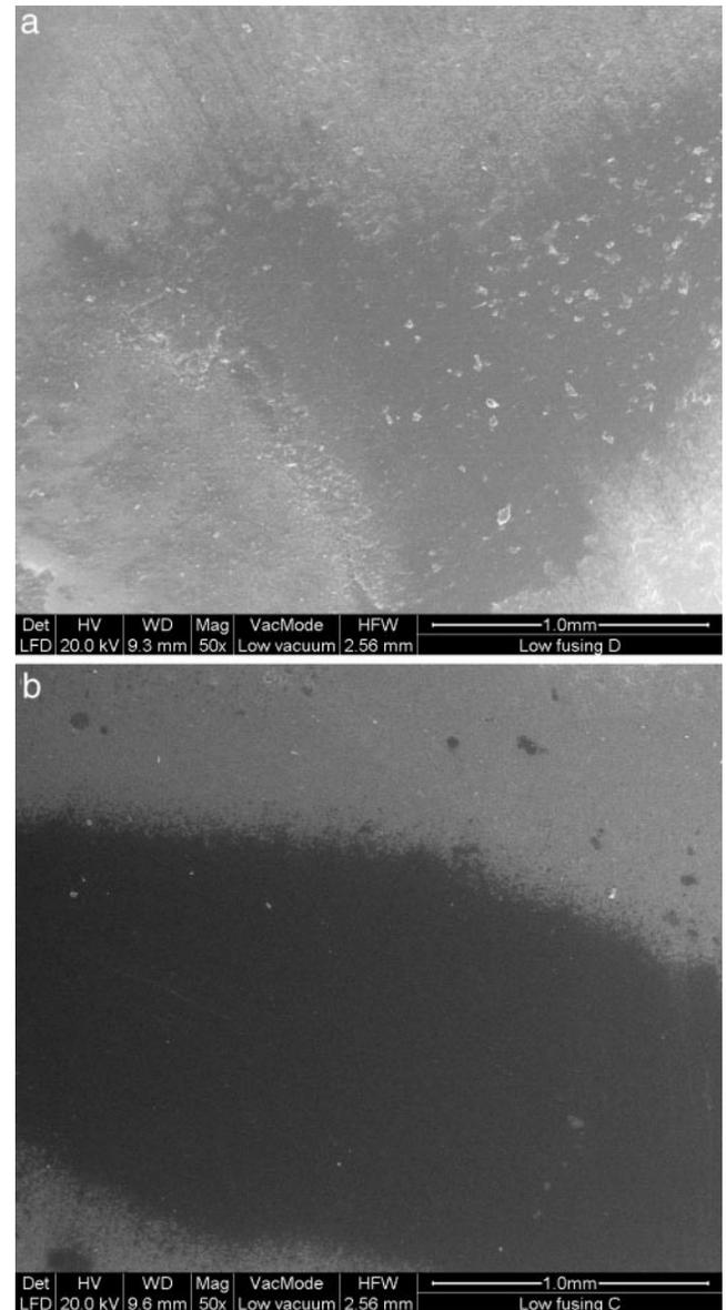
**FIGURE 2.** (a) Scanning electron microscope (SEM) image of low-fusing porcelain polished with fluted bur (50 $\times$ ). (b) SEM image of low-fusing porcelain polished with fluted bur and Sof-Lex discs (50 $\times$ ).
