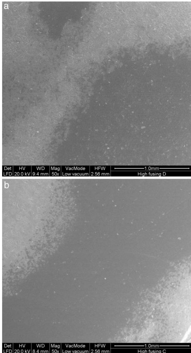
**FIGURE 1.** (a) Scanning electron microscope (SEM) image of high-fusing porcelain polished with fluted bur (50 $\times$ ). (b) SEM image of high-fusing porcelain polished with fluted bur and Sof-Lex discs (50 $\times$ ).
