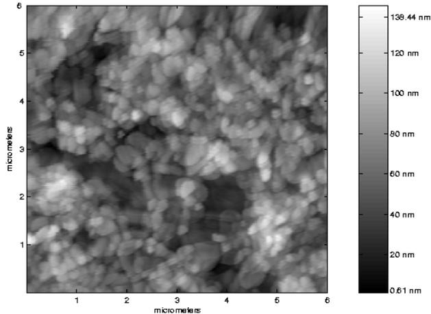
*Sample of an AFM image of gold surface (AFM data courtesy of Purdue University Nanoscale Physics Lab)*
