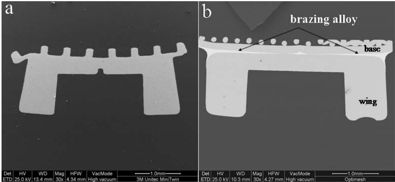
**Figure 1.** Secondary electron images from the cross sections of (a) a single-piece bracket (MIM) and (b) a bracket consisting of base and wing components joined together by a brazing alloy (indicated by the lighter zone between base and wing). Original magnification 30×.
