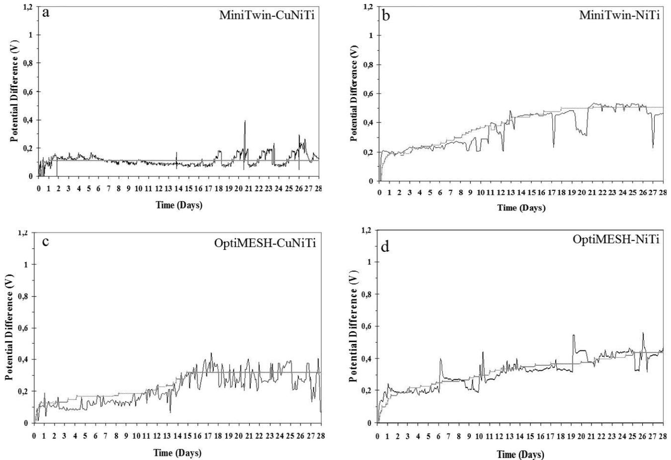
**Figure 3.** Potential difference (V) throughout duration of experiment. (a) Minitwin with CuNiTi wire; (b) Minitwin with NiTi wire; (c) OptiMESH with CuNiTi wire; and (d) OptiMESH with NiTi. Dash lines represent the trend curve among the experimental data.
