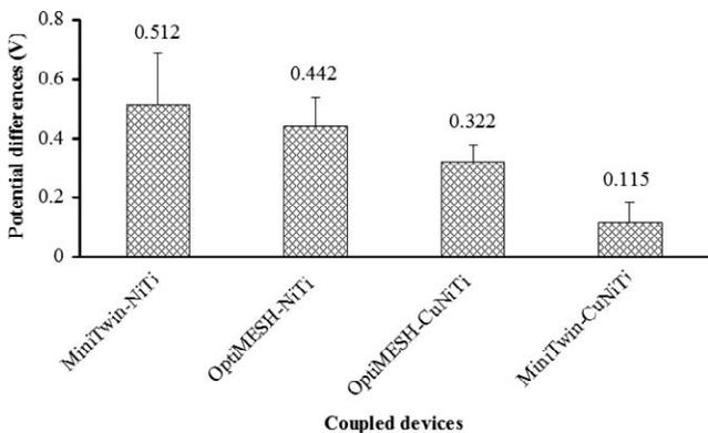
**Figure 4.** Mean values and standard deviations of potential differences after 28 days of all couples tested in lactic acid. Results are sorted in decreasing order. Only the mean values are presented above each bar.
