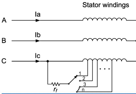
**Fig. 7.** Schematic of the tapped induction motor windings.
