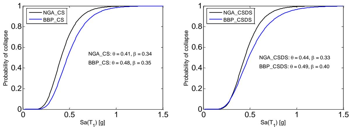
Figure 7. Collapse fragilities for ground motion sets from CS and CSDS groups,  $\lambda / \lambda_0 = 0.4$ ;  $\theta$  and  $\beta$  represent the median collapse capacity and dispersion, respectively
