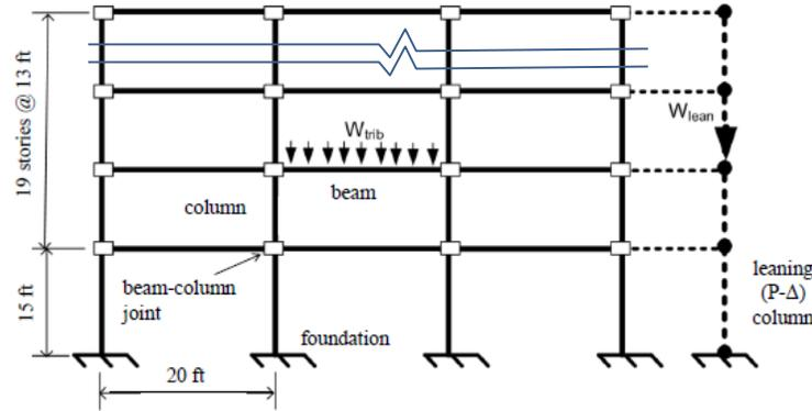
Model periods:  $T_1 = 2.63s$ ;  $T_2 = 0.85s$ ;  $T_3 = 0.45s$
