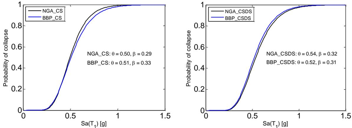
Figure 7. Collapse fragilities for ground motion sets from CS and CSDS groups,  $\lambda / \lambda_0 = 1.0$ ;  $\theta$  and  $\beta$  represent the median collapse capacity and dispersion, respectively
