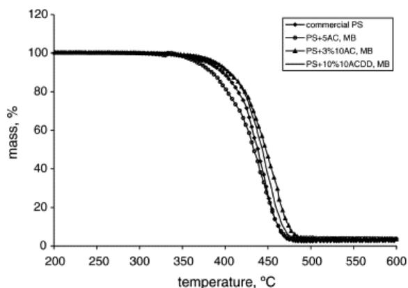
Fig. 12. TGA analysis for nanocomposites prepared melt blending.
