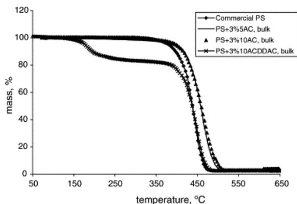
Fig. 11. TGA analysis for nanocomposites prepared by bulk polymerisation.
