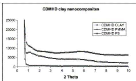
Fig. 8. XRD for CDMHCL and its nanocomposites.
