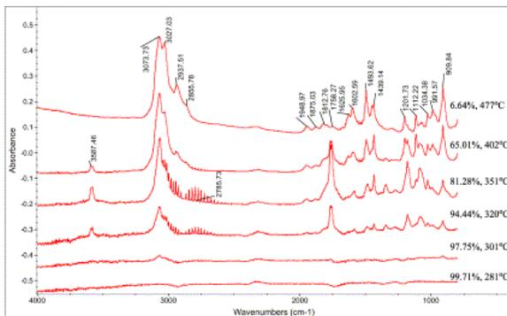
Fig. 6. Infrared spectra of the evolved gases as a function of temperature for CTPP.
