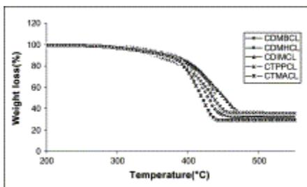
Fig. 7. TGA for PS surfactant modified clays.
