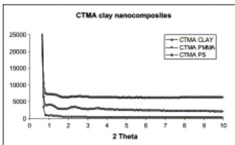
Fig. 10. XRD for CTMACL and its nanocomposites.
