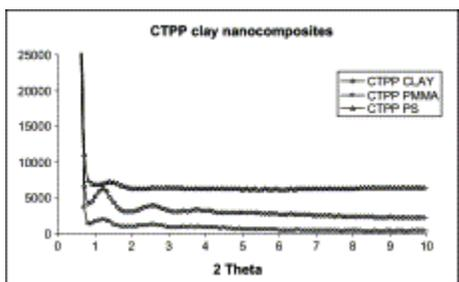
Fig. 12. XRD for CTPPCL and its nanocomposites.
