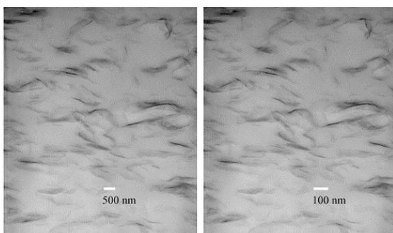
Fig. 13. TEM images of CDMHCL–PMMA nanocomposite at low magnification (left) and high magnification (right).
