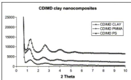
Fig. 11. XRD for CDMIDCL and its nanocomposites.
