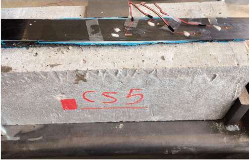
Figure 7. FRP debonding failure of pull-out specimen CS5.
