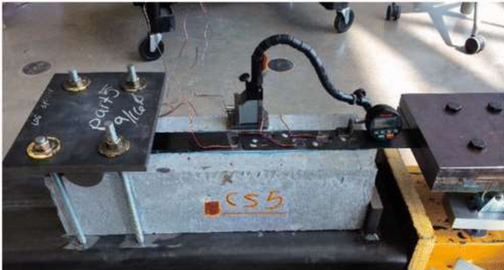
Figure 6. Application of digital dial gauge to obtain the relative slip at the precrack tip.
