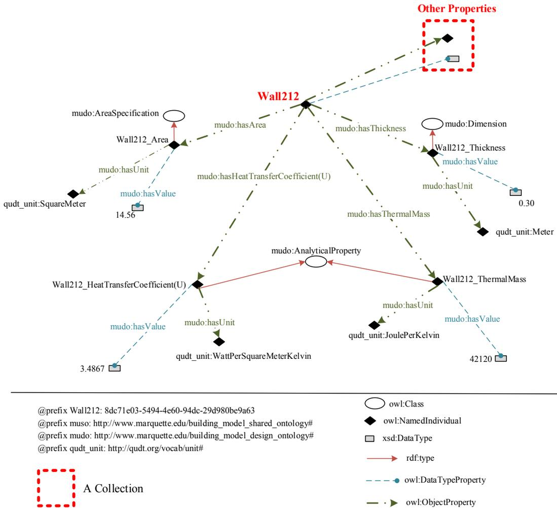
**Fig. 4. Wall212 properties in the BIM knowledge base**
