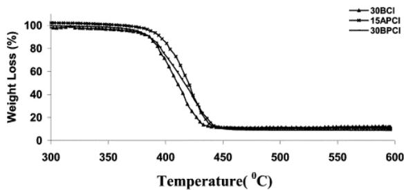
Fig. 9. TGA curve of PCL/clay hybrids.
