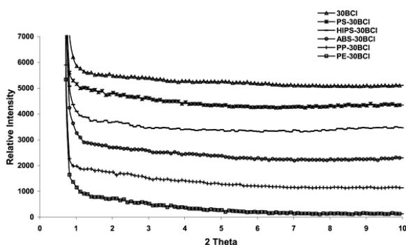
Fig. 2. XRD patterns of polymer/30BCL nanocomposites.
