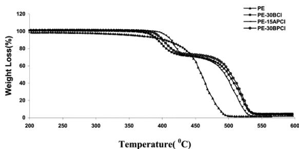
Fig. 14. TGA curve of PE-PCL/clay nanocomposites.
