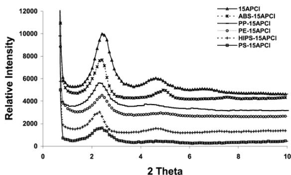
Fig. 4. XRD patterns of polymer/15APCL nanocomposites.
