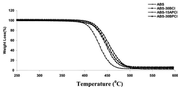
Fig. 12. TGA curve of ABS-PCL/clay nanocomposites.
