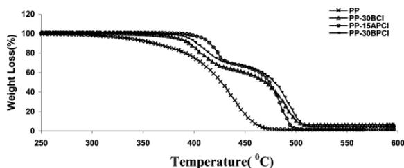
Fig. 13. TGA curve of PP-PCL/clay nanocomposites.
