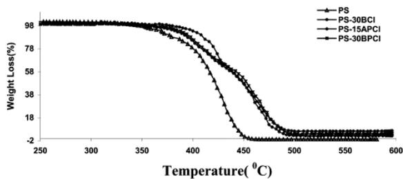
Fig. 10. TGA curve of PS-PCL/clay nanocomposites.
