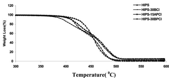
Fig. 11. TGA curve of HIPS-PCL/clay nanocomposites.
