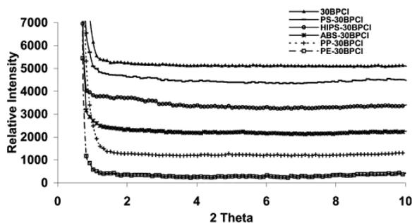
Fig. 3. XRD patterns of polymer/30BPCL nanocomposites.
