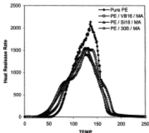
Fig. 10. Comparison of the heat release rate (HRR) plots for pure PE and PE/MA/clay nanocomposites at 35 Kw/m<sup>2</sup> heat flux.
