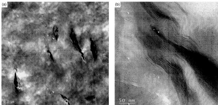
Fig. 4. TEM images of PE/MA/Si18 at (a) low magnification and (b) high magnification.
