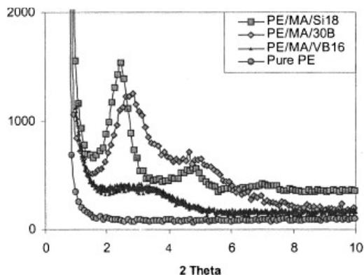
Fig. 2. X-ray diffraction pattern of PE/MA/clay nanocomposites.
