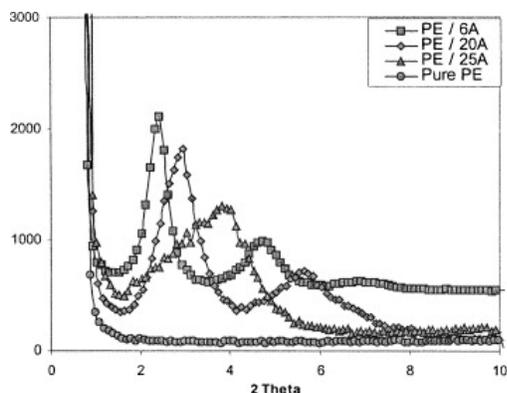
Fig. 1. X-ray diffraction pattern of PE/clay nanocomposites.
