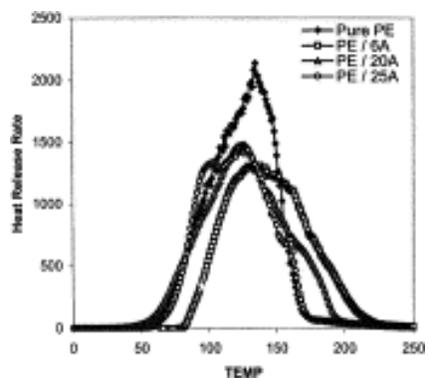
Fig. 9. Comparison of the heat release rate (HRR) plots for pure PE and PE/clay nanocomposites at 35 Kw/m<sup>2</sup> heat flux.
